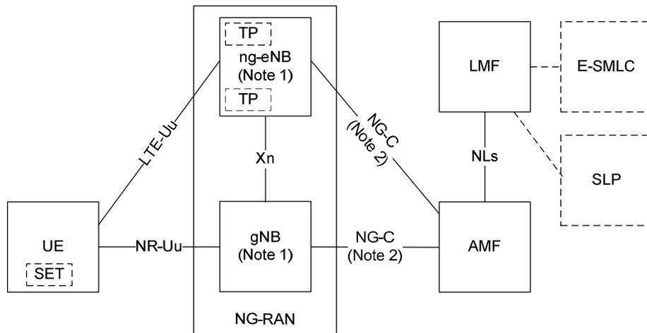
**Figure 5.1-1: UE Positioning Architecture applicable to NG-RAN**
