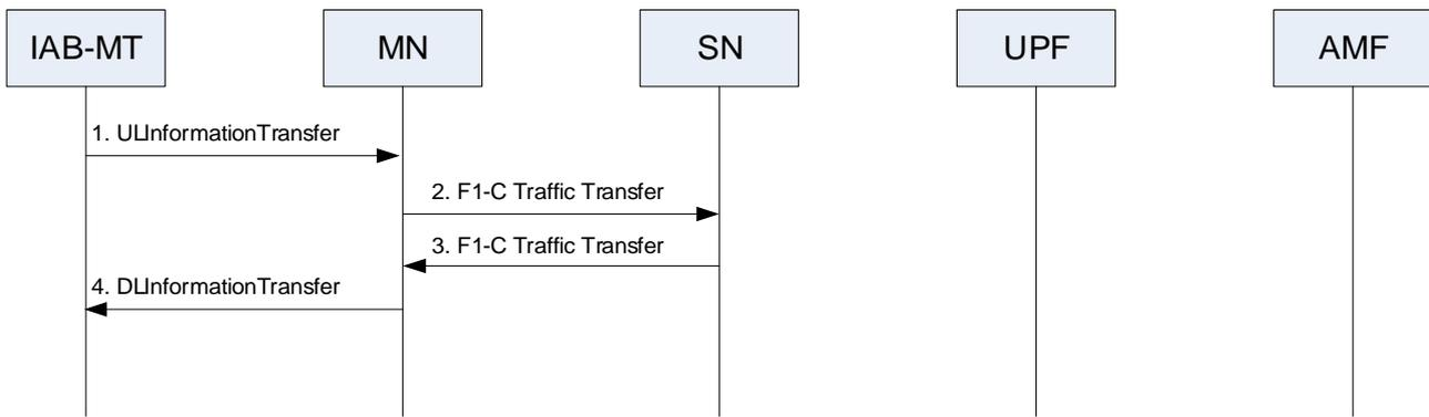
**Figure 10.15-2: Scenario 1: F1-C transfer between IAB-MT and SN (F1-terminating node) in NR-DC**
