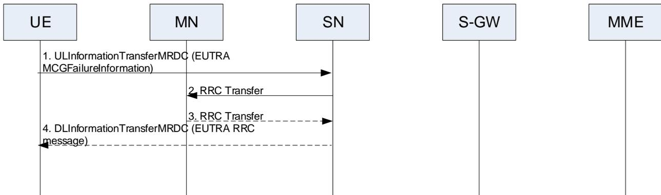
**Figure 10.10.1-4: RRC Transfer procedure for MCG failure information**
