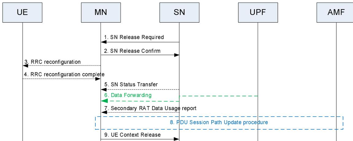
**Figure 10.4.2-2: SN release procedure - SN initiated**
