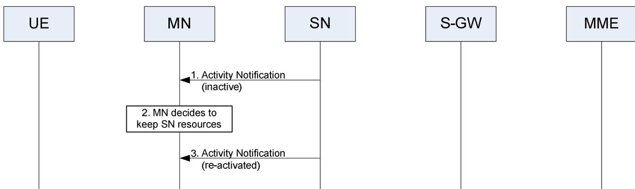
**Figure 10.12.1-1: Support of Activity Notification in EN-DC**
