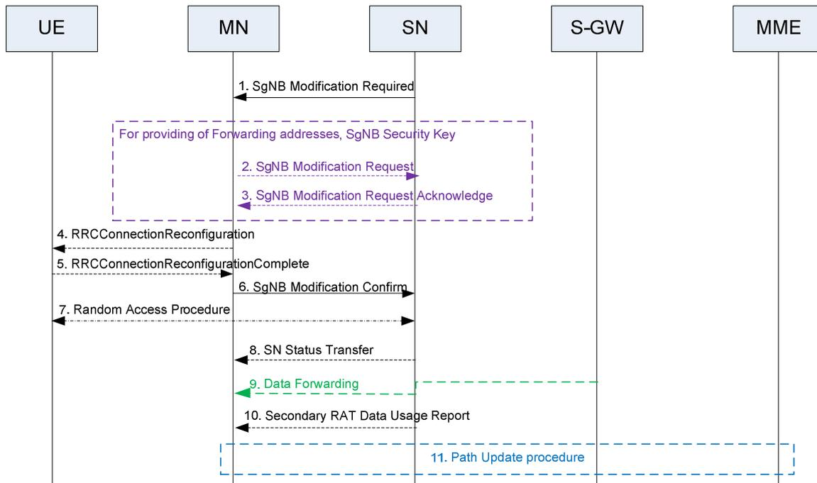
**Figure 10.3.1-2: SN Modification procedure - SN initiated with MN involvement**
