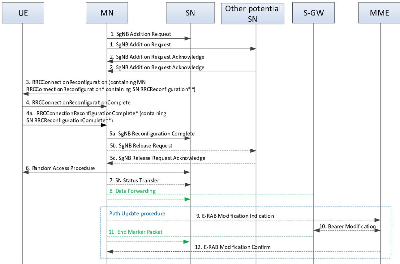
**Figure 10.2.1-2: Conditional Secondary Node Addition procedure**
