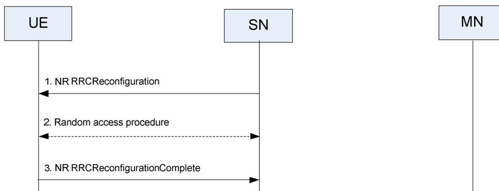
Figure 10.3.1-3: SN modification - SN initiated without MN involvement
