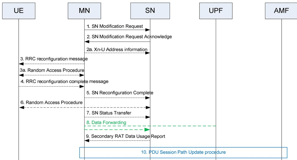
Figure 10.3.2-1: SN Modification procedure - MN initiated
