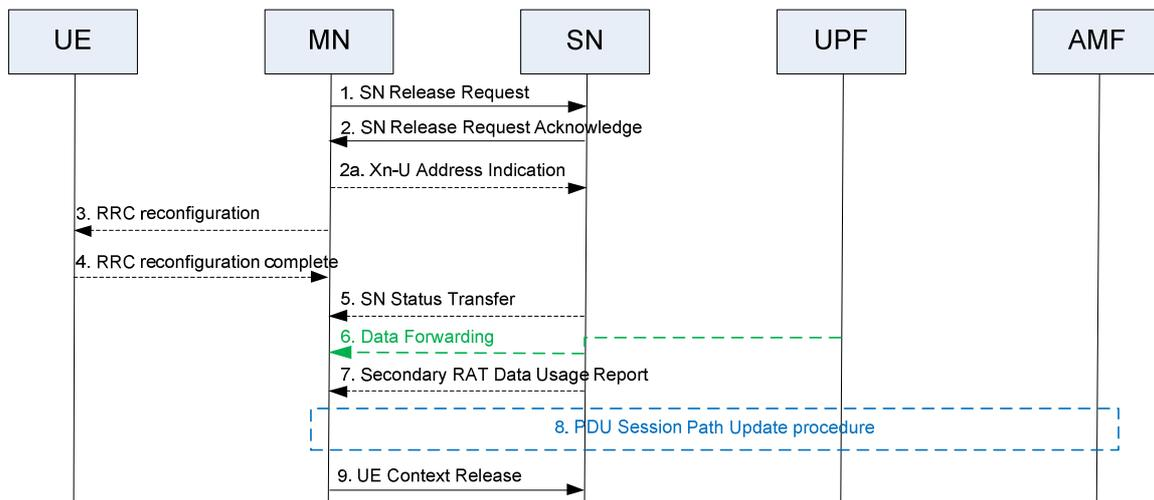
**Figure 10.4.2-1: SN release procedure - MN initiated**
