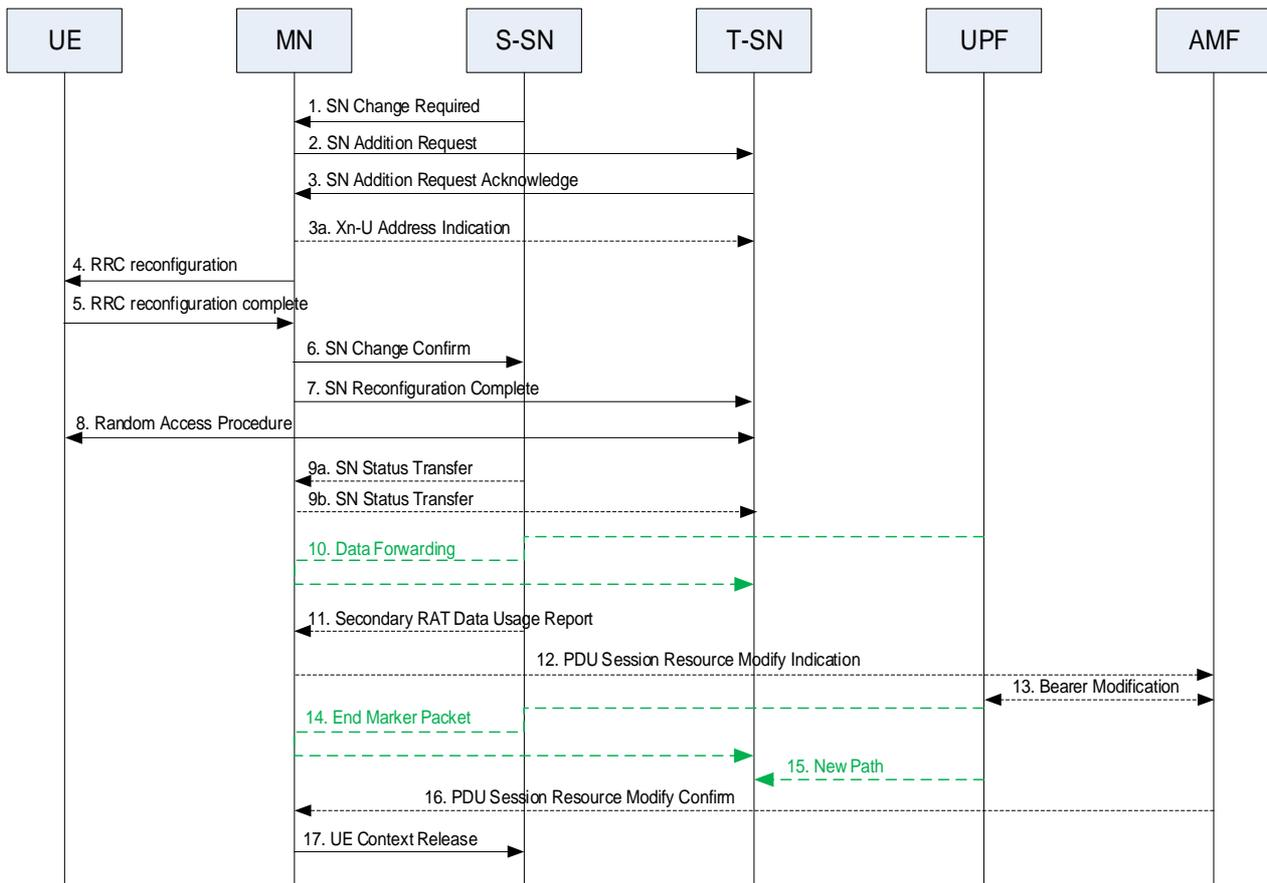
**Figure 10.5.2-2: SN change procedure - SN initiated**
