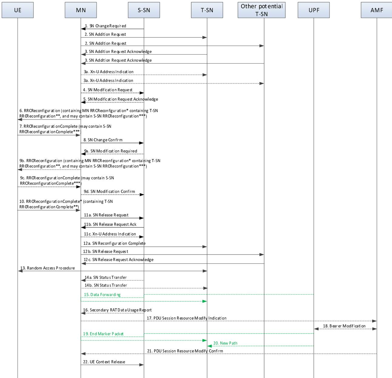
Figure 10.5.2-4: Conditional SN change procedure - SN initiated
