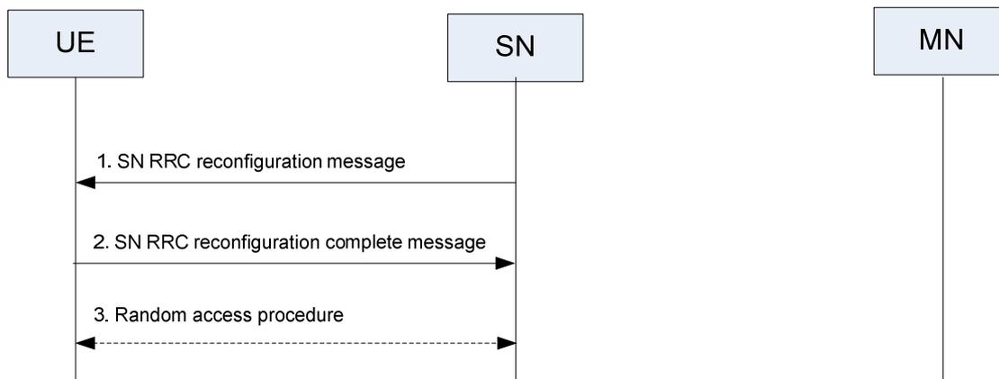
**Figure 10.3.2-3: SN Modification – SN initiated without MN involvement**
