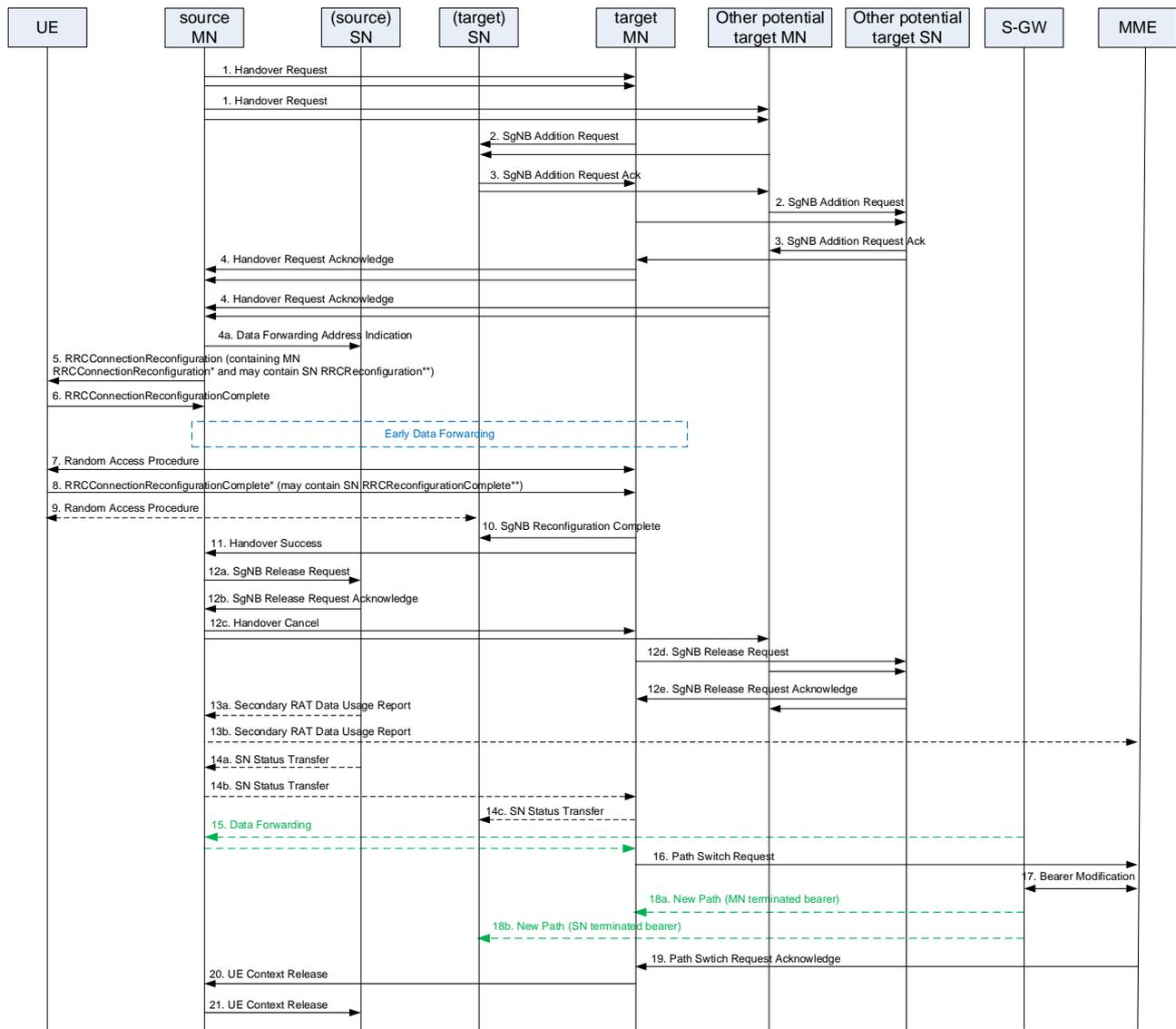
Figure 10.19.1-1: Conditional Handover with Secondary Node procedure
