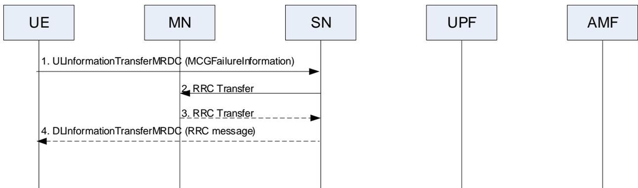
**Figure 10.10.2-4: RRC Transfer procedure for MCG failure information**
