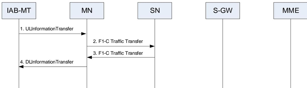
**Figure 10.15-1: F1-C transfer procedure in EN-DC**
