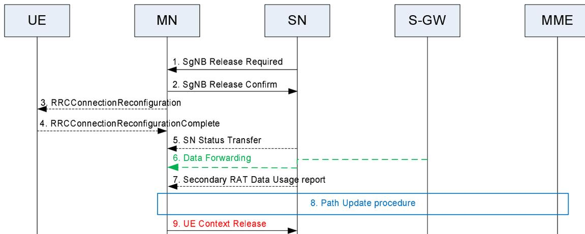
**Figure 10.4.1-2: SN Release procedure – SN initiated**
