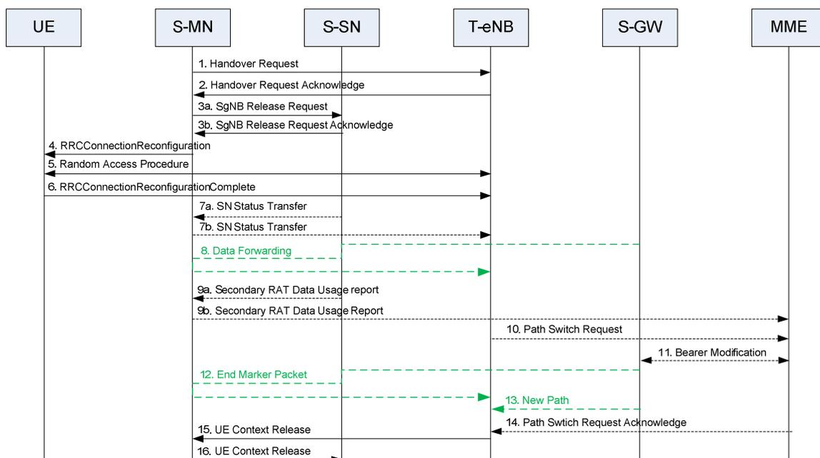
Figure 10.8.1-1: Master Node to eNB Change procedure
