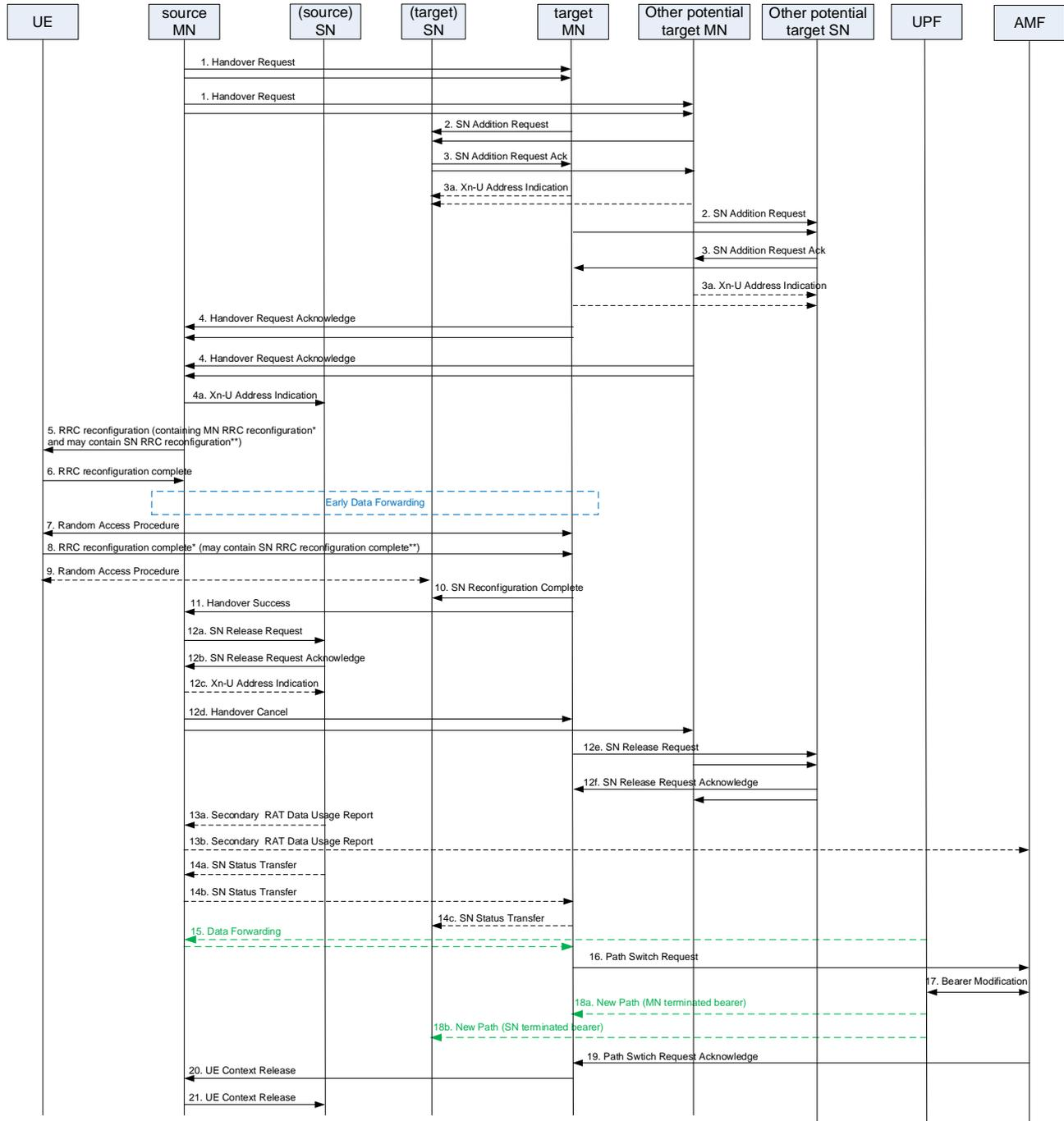
**Figure 10.19.2-1: Conditional Handover with Secondary Node procedure**
