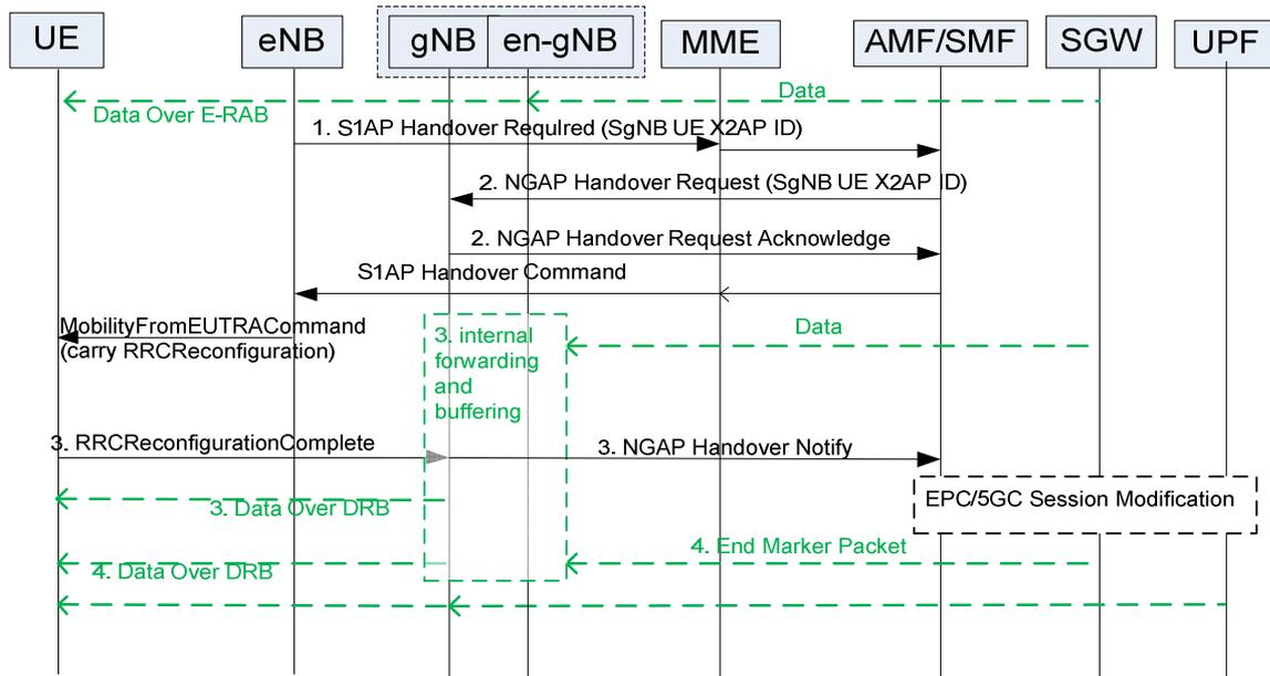
**Figure 10.16.2-1: Inter-system handover from EPS to 5GS with the Secondary Node used as target**
