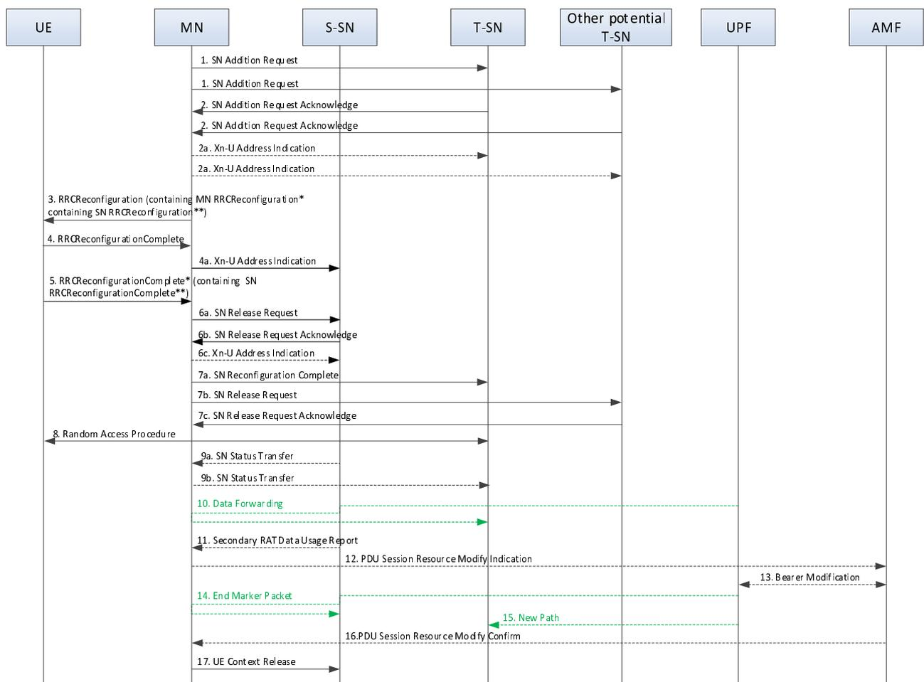
Figure 10.5.2-3: Conditional SN change procedure - MN initiated
