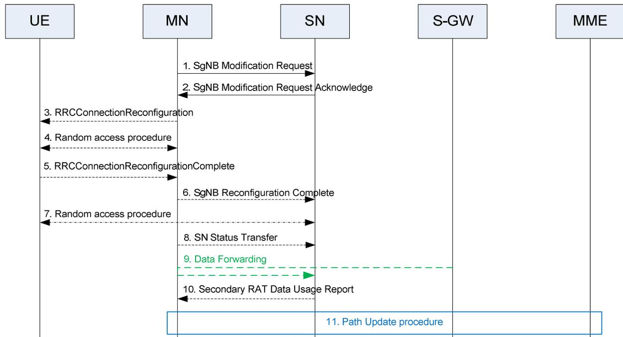
**Figure 10.3.1-1: SN Modification procedure - MN initiated**
