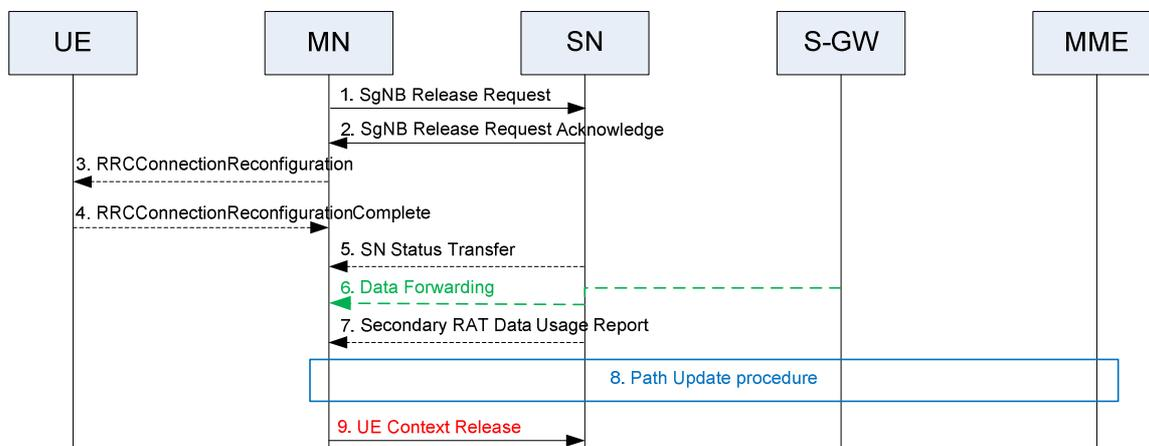
**Figure 10.4.1-1: SN Release procedure – MN initiated**
