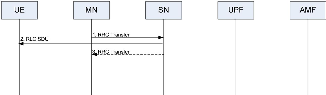
**Figure 10.10.2-1: RRC Transfer procedure for split SRB (DL operation)**
