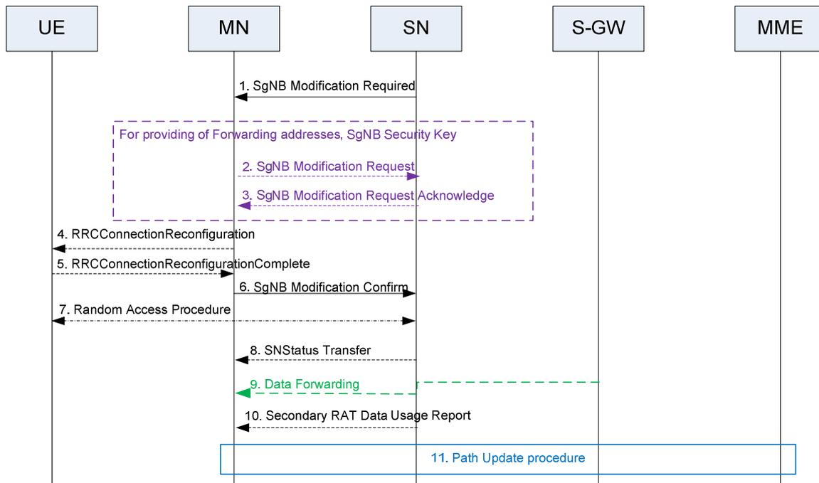
**Figure 10.3.1-2: SN Modification procedure - SN initiated with MN involvement**
