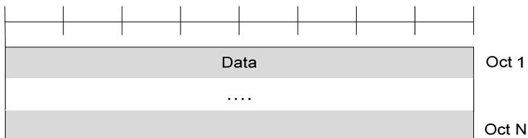
Figure 6.2.2.1-1: SDAP Data PDU format without SDAP header
