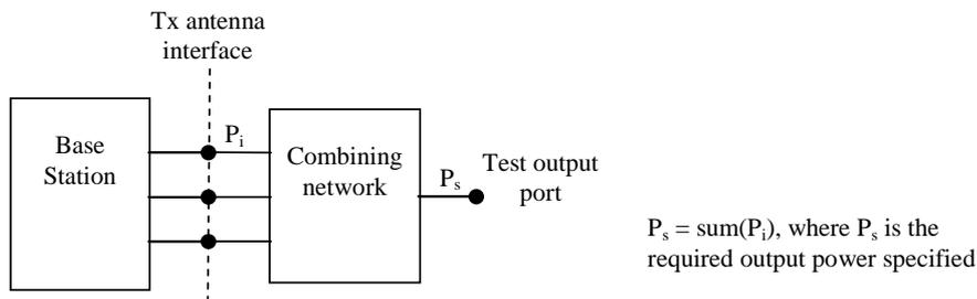
**Figure 4.10.7.2-1: Transmitter test set-up**
