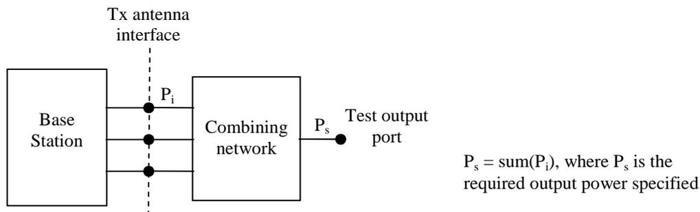
**Figure 4.10.7.2-1: Transmitter test set-up**
