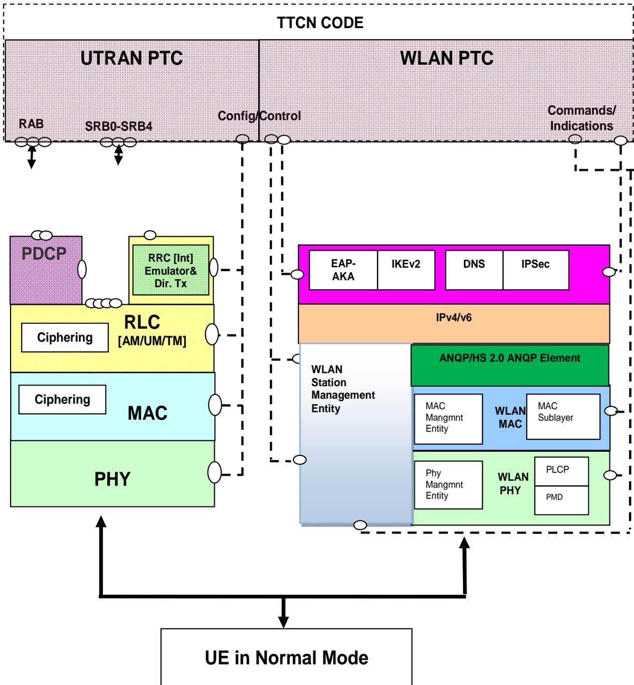
Figure 4.4.6.2-1: Test model for UTRAN-WLAN interworking testing
