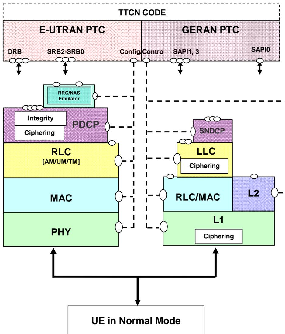
Figure 4.4.2-1: Test model for Inter RAT E-UTRAN-GERAN testing
