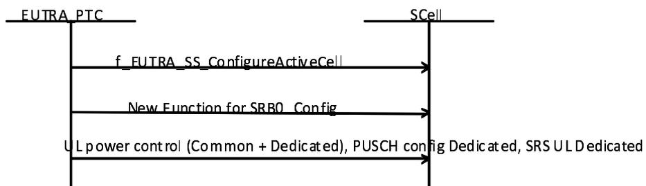
**Figure 7.24.2-1: CA sequence of an initial cell configuration for a cell to be used as SCell**
