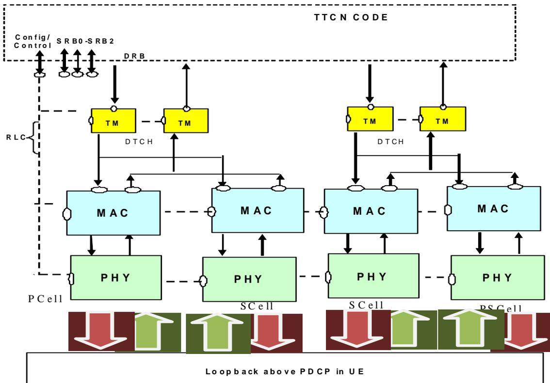
**Figure 4.2.4B.1-1: Test model for DC MAC testing**
