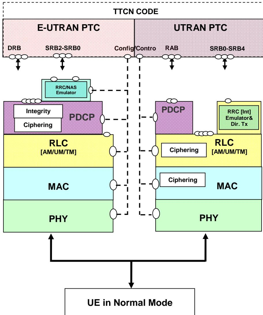
Figure 4.4.1-1: Test model for Inter RAT E-UTRAN-UTRAN testing
