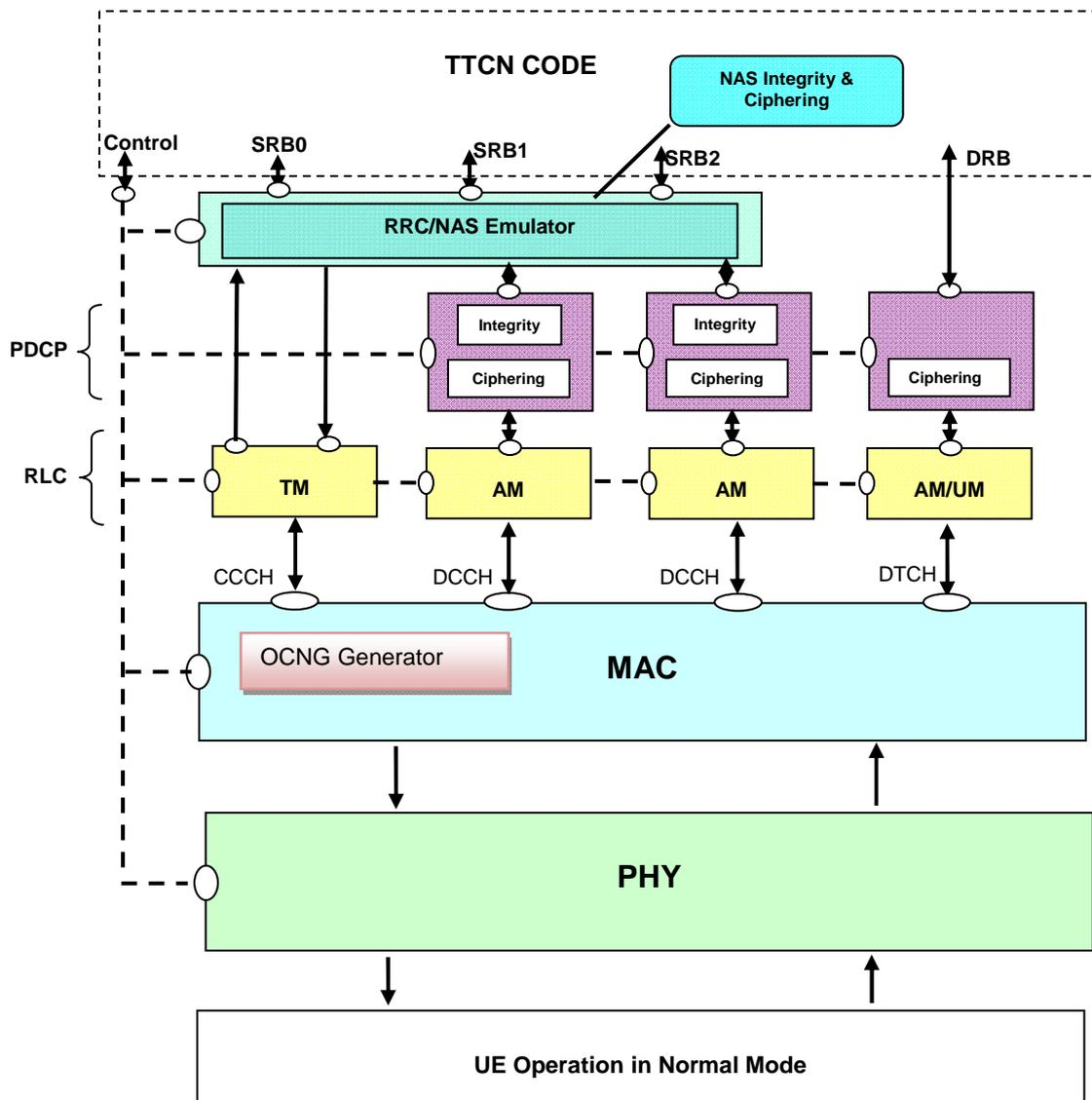
Figure 4.2.8-1: Test model for testing with OCNG
