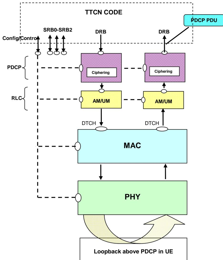
Figure 4.2.1.3.2-1: Test model for PDCP (Non ROHC) testing
