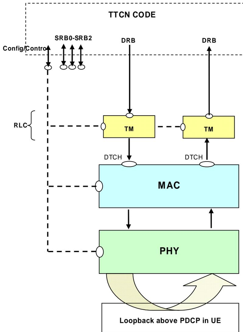
Figure 4.2.1.2.3-1: Test model for RLC AM/UM testing
