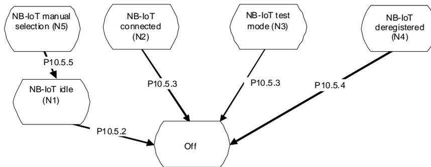
Figure 10.5.1-1: UE postamble states and procedures for NB-IoT
