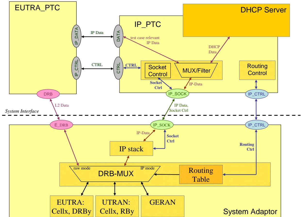
Figure 4.2.4.1-1: Example of EUTRA IP test model with a DHCP server
