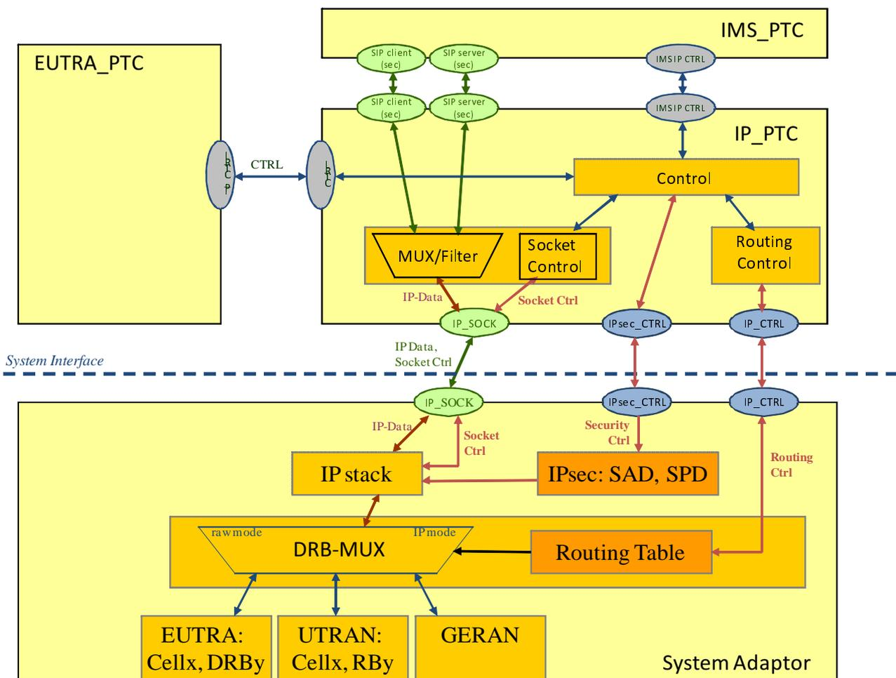
Figure 4.2.5-1: Example for IP model supporting IMS
