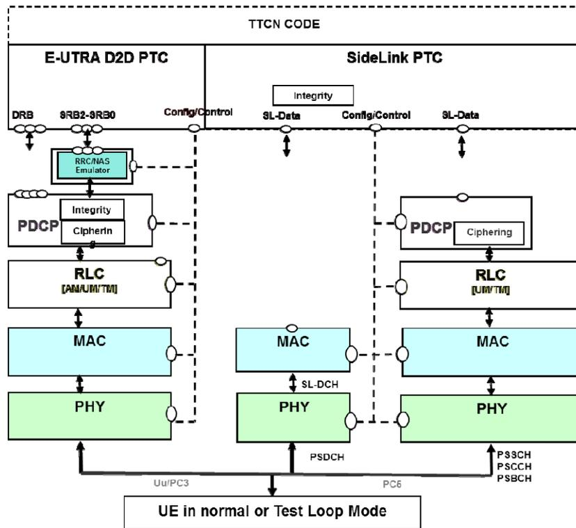
Figure 4.2.9-1: D2D ProSe test model
