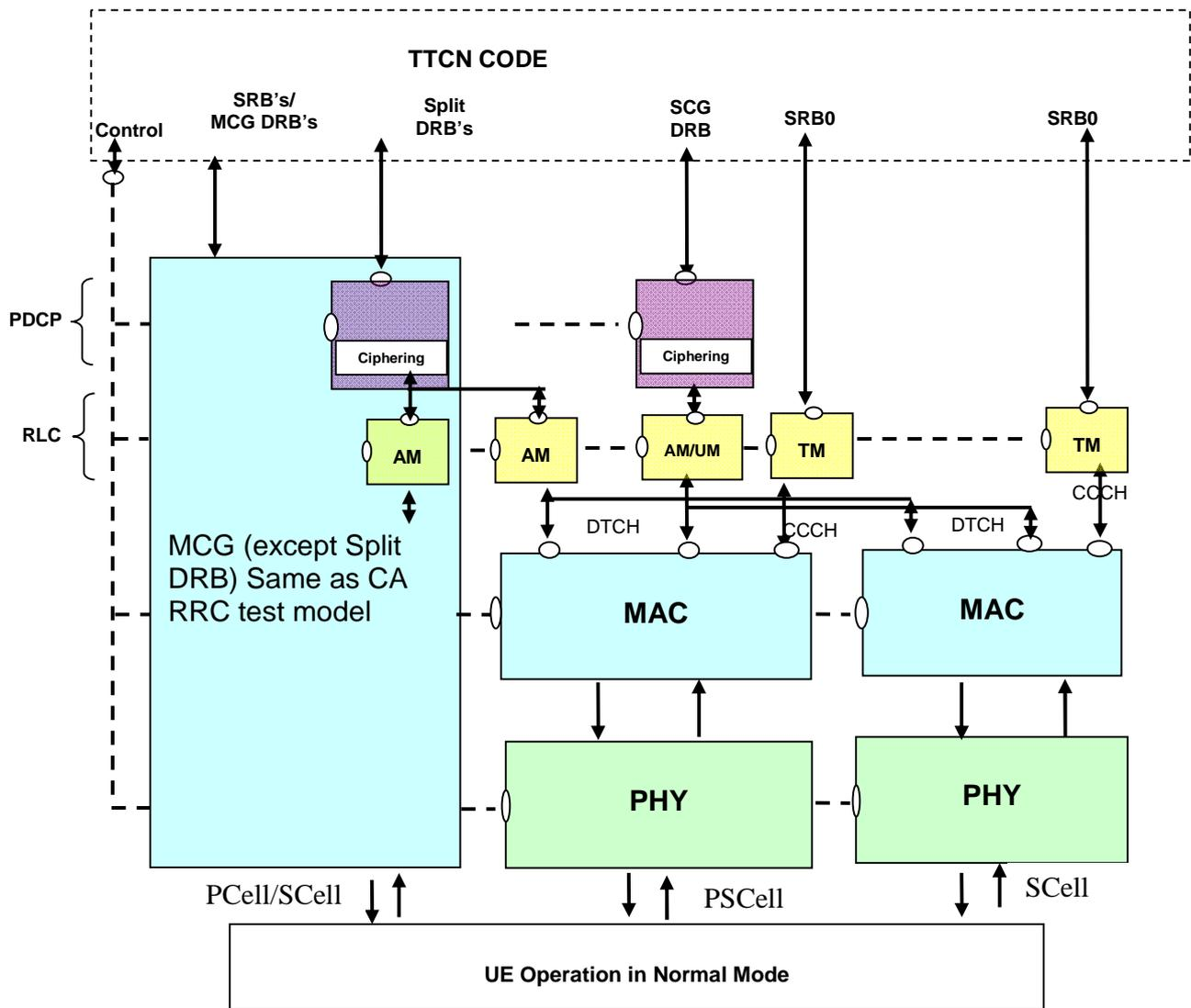
Figure 4.2.4B.3-1: Test model for DC RRC testing
