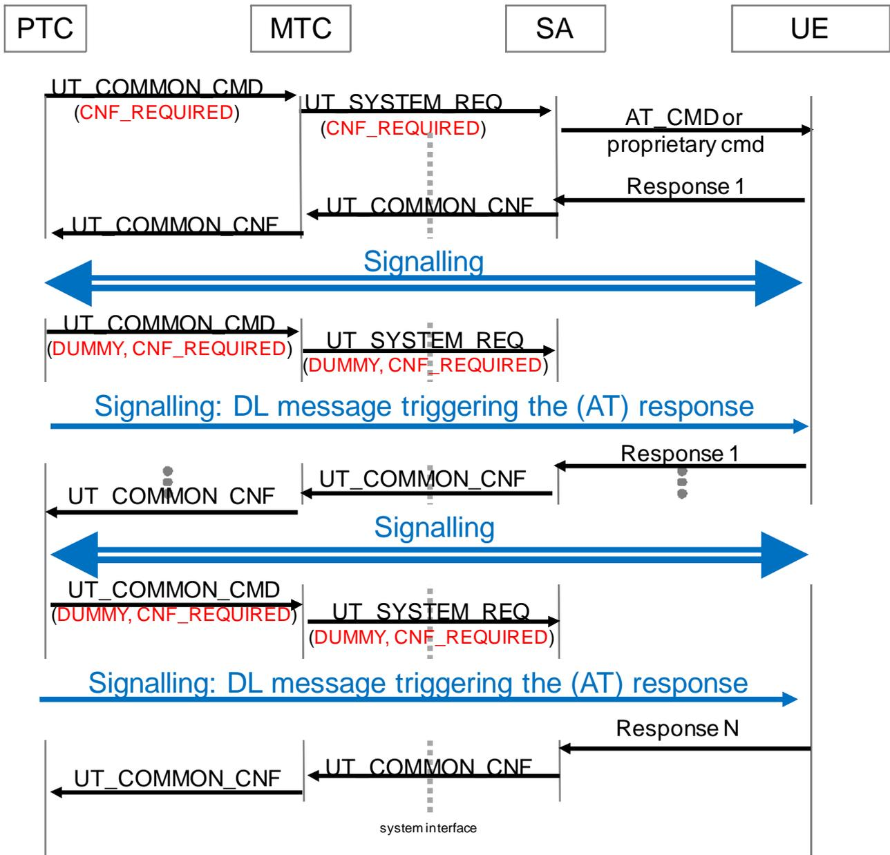
Figure E.4-1: Multiple responses (automatic operation)
