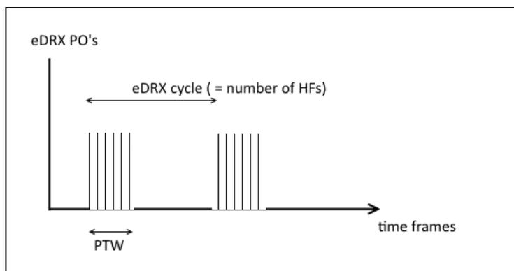
**Figure 7.7.3.1.1-1: Paging cycles in eDRX idle mode**
