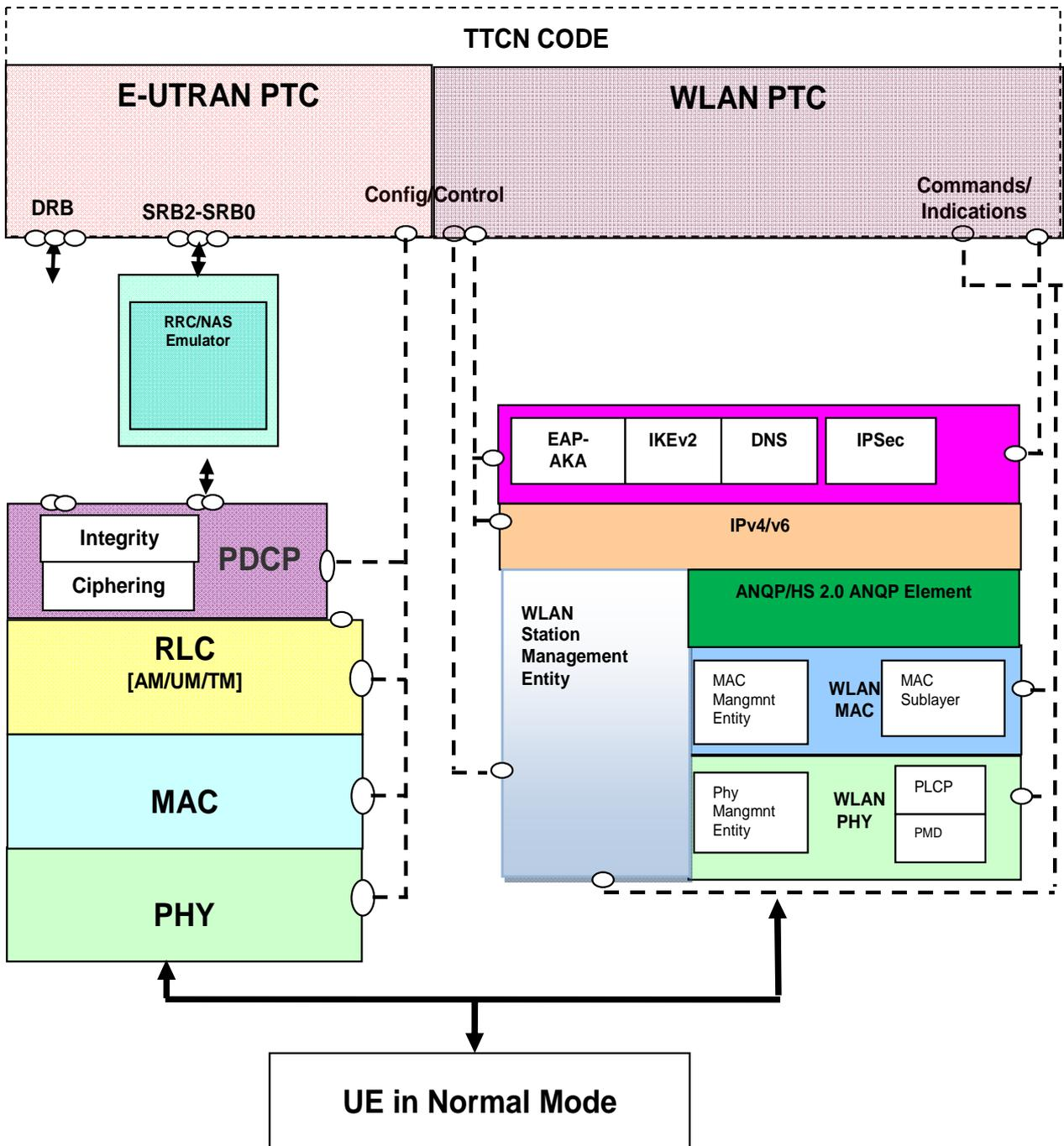
Figure 4.4.6.1-1: Test model for E-UTRAN-WLAN interworking testing
