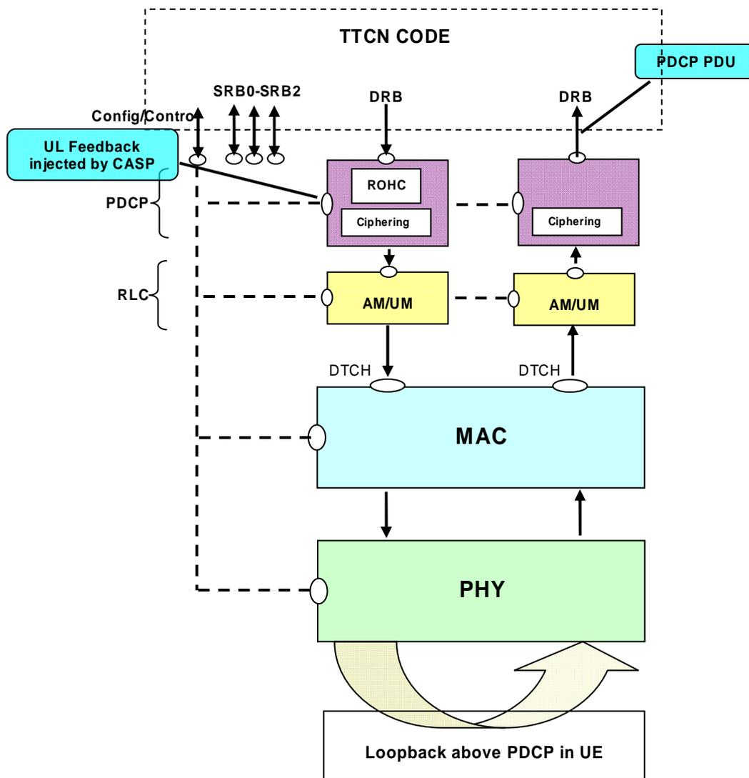
Figure 4.2.1.3.1-1: Test model for PDCP ROHC testing
