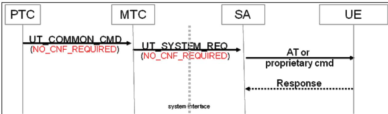
Figure E.1-1: No confirmation (automatic operation)
