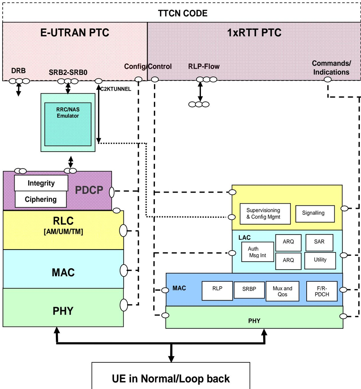
Figure 4.4.3.2-1: Test model for InterRAT E-UTRAN-CDMA2000 1xRTT testing
