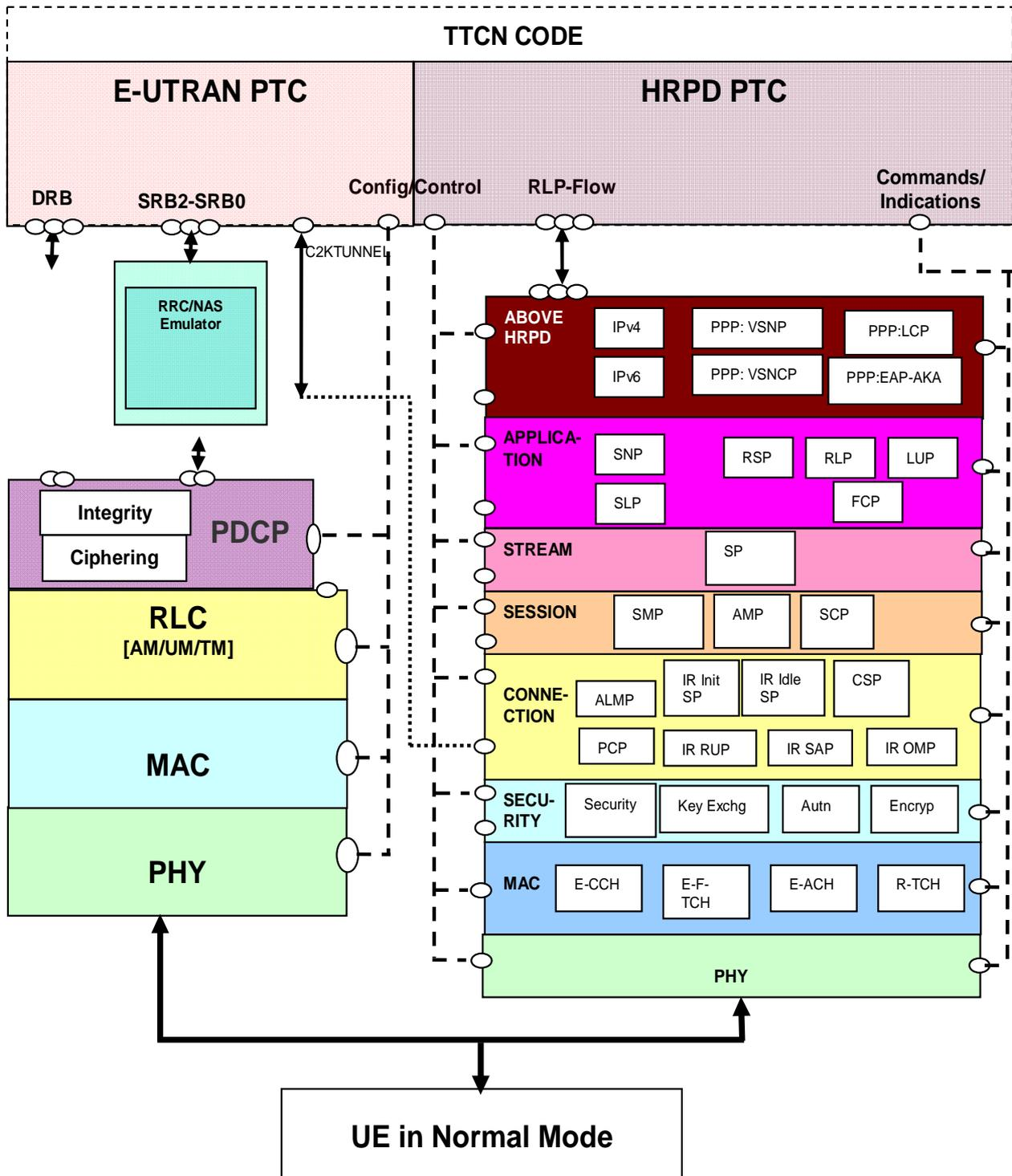
Figure 4.4.3-1: Test model for InterRAT E-UTRAN-CDMA2000 HRPD testing
