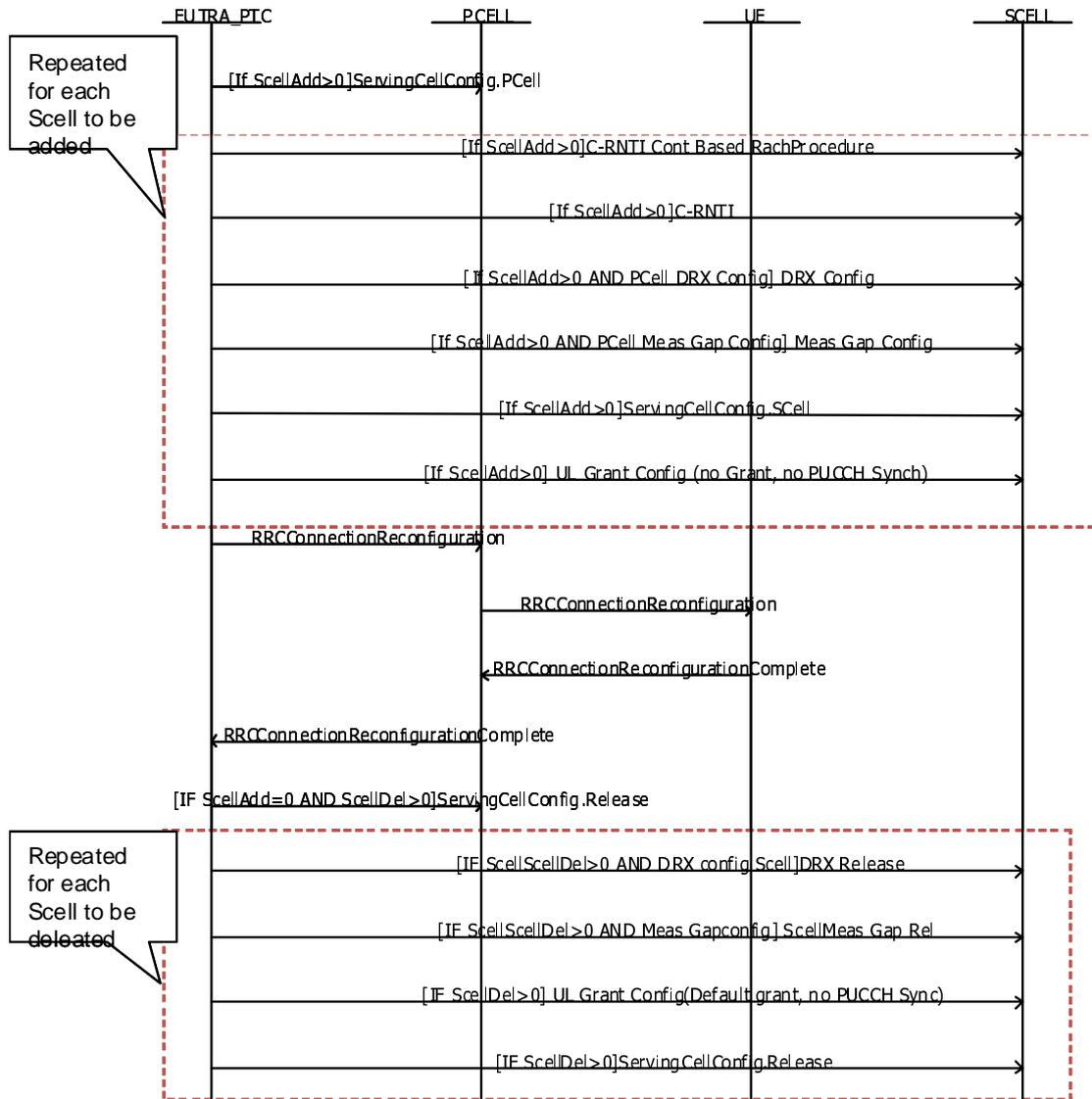
Figure 7.24.3-1: CA sequence of Scell Addition and/or release
