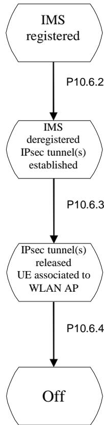
Figure 10.6.1-1: UE postamble states and procedures for WLAN
