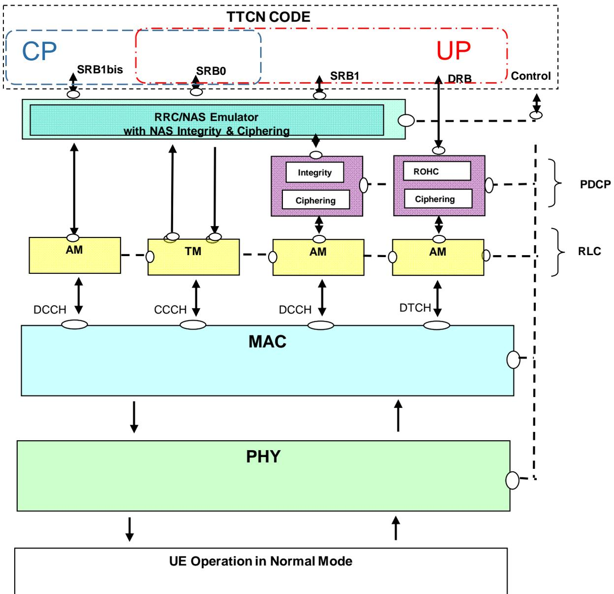
**Figure 4A.2.2-1: Test model for NB-IoT RRC/NAS testing**
