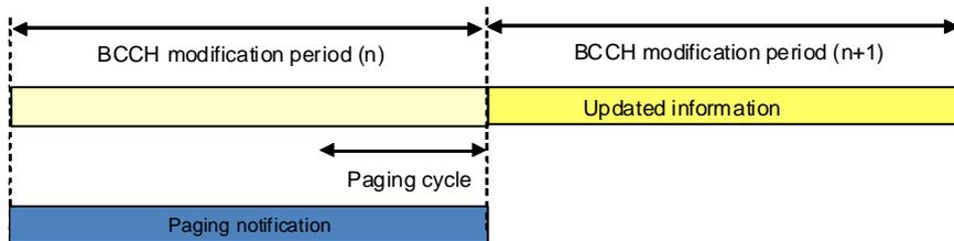
Figure 7.7.3.1.2-1: Paging notification UE in connected mode
