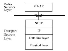
Figure 4.1.1: M2 signalling bearer protocol stack
