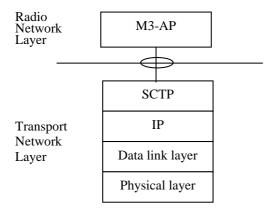
Figure 5.1.1: M3 signalling bearer protocol stack
