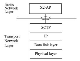
Figure 4.1: X2 signalling bearer protocol stack
