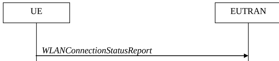
Figure 5.6.15.2.1-1: WLAN connection status reporting
