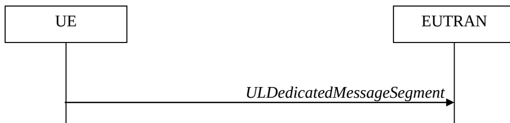
Figure 5.6.22.1-1: UL message segment transfer
