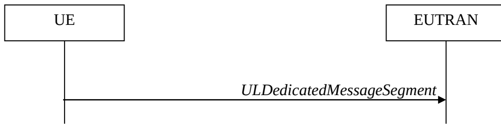
Figure 5.6.22.1-1: UL message segment transfer
