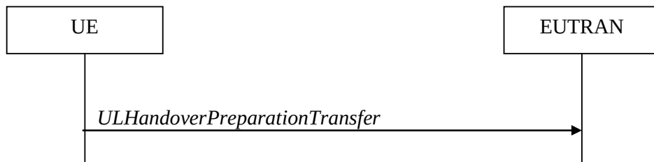
Figure 5.4.5.1-1: UL handover preparation transfer
