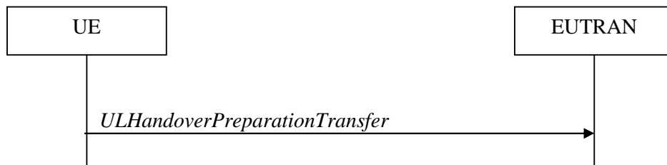
Figure 5.4.5.1-1: UL handover preparation transfer
