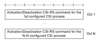
Figure 6.1.3.14-1: Activation/Deactivation of CSI-RS resources MAC Control Element
