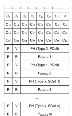
Figure 6.1.3.6a2-4: Extended PHR MAC Control Element supporting 32 serving cells with configured uplink
