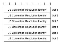
Figure 6.1.3.4-1: UE Contention Resolution Identity MAC control element
