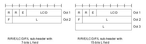
Figure 6.1.6-1: R/R/E/LCID/F/L MAC subheader
