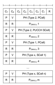
Figure 6.1.3.6a1-3: Extended PHR MAC Control Element supporting PUCCH on SCell
