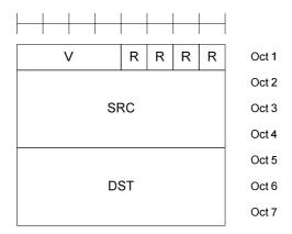
Figure 6.1.6-3a: SL-SCH MAC subheader for V="0011"
