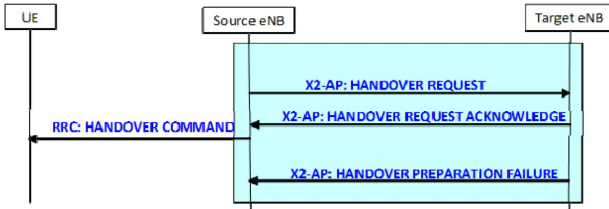
Figure 20.2.2.1-1: Handover Preparation procedure
