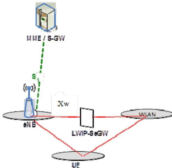
Figure 22A.3-1: LWIP Overall Architecture
