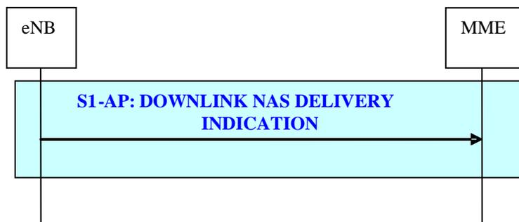
**Figure 19.2.2.6-5: Downlink NAS Delivery Indication procedure**
