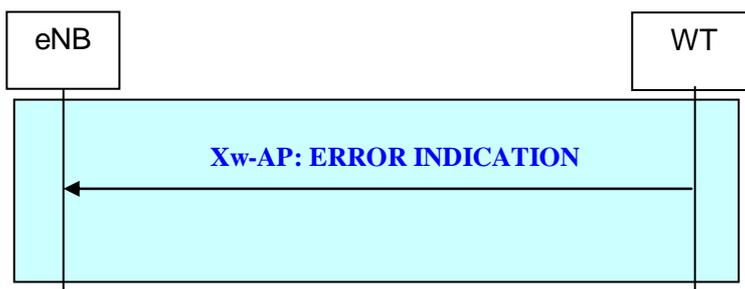
Figure 22B.2.2.11.1-1: Error Indication procedure initiated by WT
