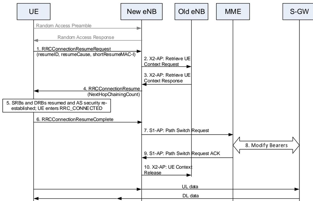
**Figure 7.3a.3-3: RRC Connection Resume procedure in different eNB**
