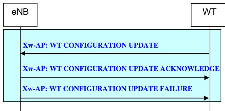
**Figure 22B.2.2.10-1: WT Configuration Update procedure**
