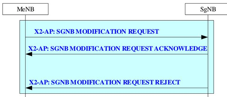
**Figure 20.2.2.22-1: MeNB initiated SgNB Modification Preparation procedure**
