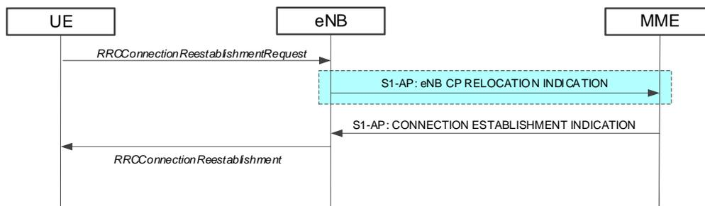
Figure 19.2.2.30-1: eNB CP Relocation Indication procedure (highlighted in blue)
