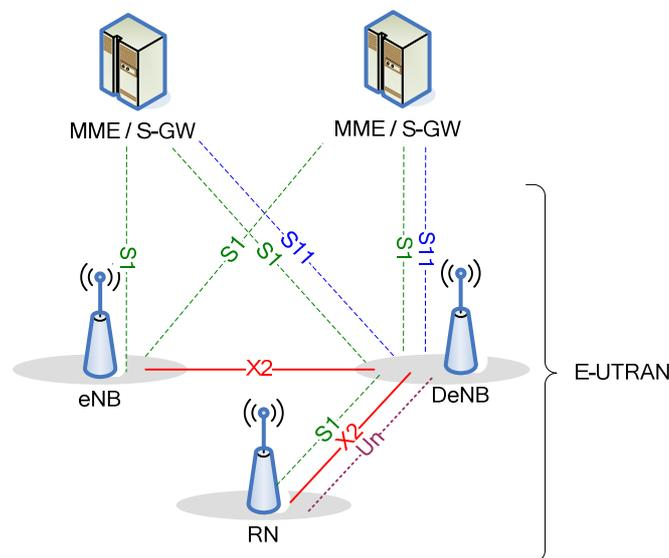
**Figure 4.7.2-1: Overall E-UTRAN Architecture supporting RNs**
