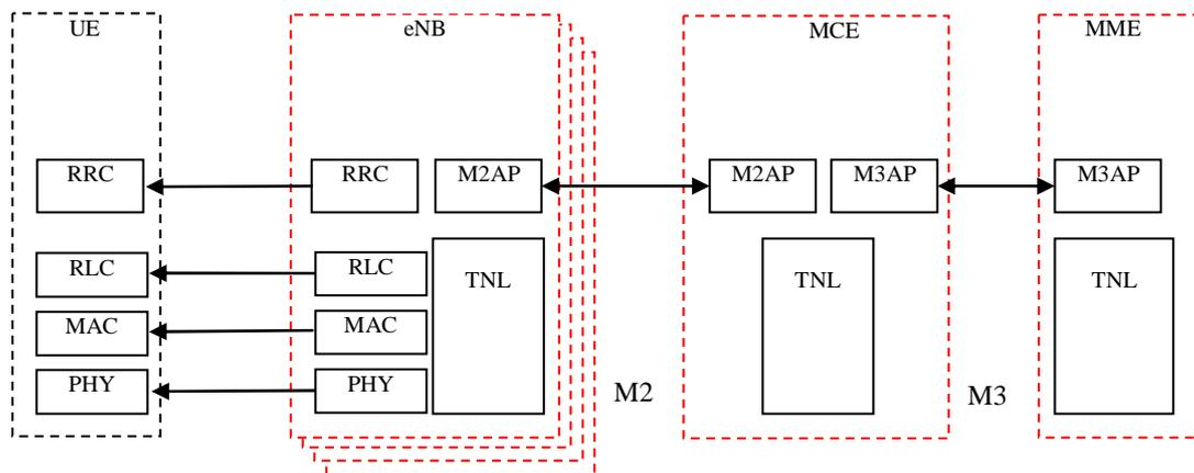
**Figure 15.1.3-1: The E-MBMS c-plane architecture**
