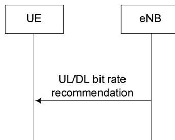
Figure 23.15.1-1: UL or DL bit rate recommendation
