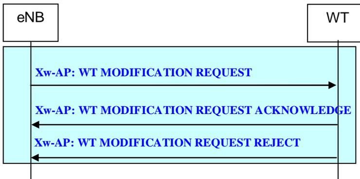
**Figure 22B.2.2.3-1: eNB initiated WT Modification Preparation procedure**
