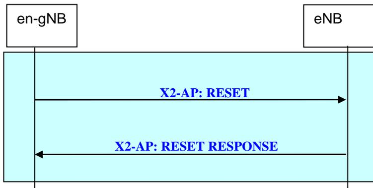
Figure 20.2.2.9-3: en-gNB-initiated Reset procedure between en-gNB and eNB
