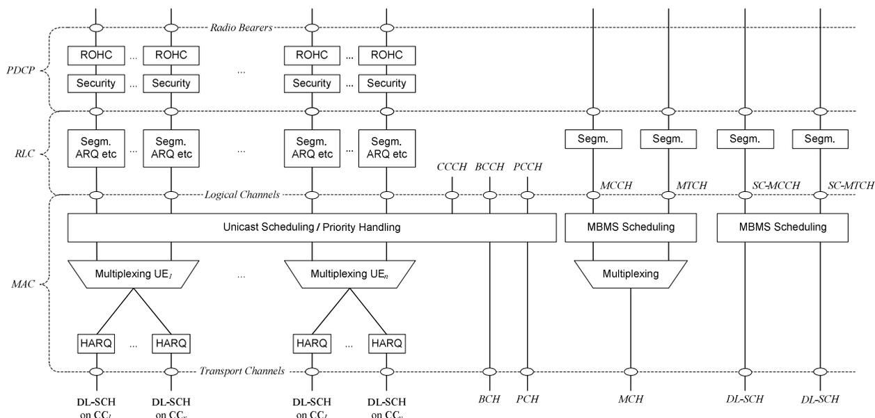
Figure 6.4-1: Layer 2 Structure for DL with CA configured
