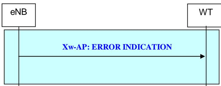
Figure 22B.2.2.11.2-1: Error Indication procedure initiated by eNB
