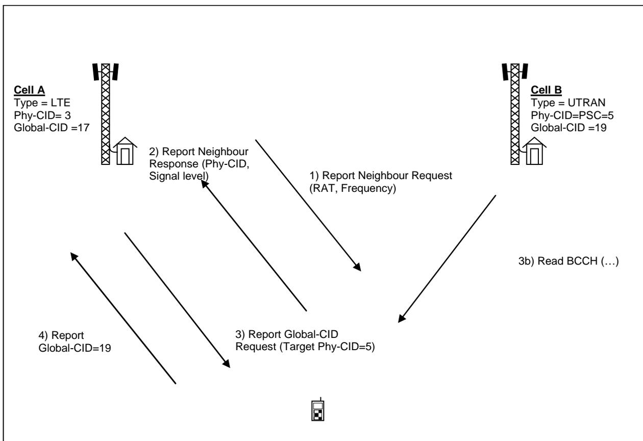
**Figure 22.3.4-1: Automatic Neighbour Relation Function in case of e.g. UTRAN detected cell**
