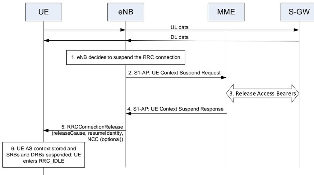
Figure 7.3a.3-1: RRC Connection Suspend procedure
