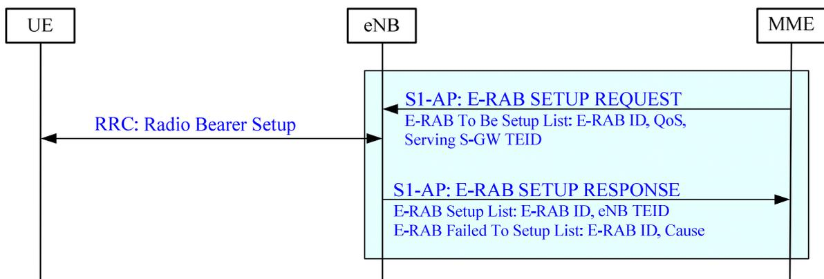
Figure 19.2.2.4.1-1: E-RAB Setup procedure
