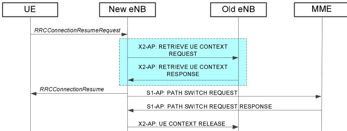
**Figure 20.2.2.19-1: Retrieve UE Context procedure (highlighted in blue) for cases of UE context resumption. Successful case**
