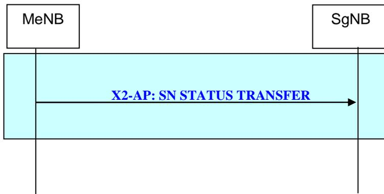
Figure 20.2.2.4-2: MeNB-initiated SN Status Transfer procedure for EN-DC.
