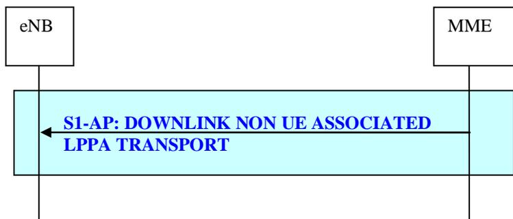
Figure 19.2.2.18.3-1: Downlink Non UE Associated LPPa Transport procedure
