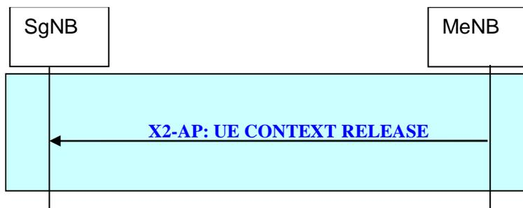
Figure 20.2.2.3-2: UE Context Release procedure for EN-DC.
