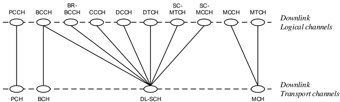
**Figure 6.1.3.2-1: Mapping between downlink logical channels and downlink transport channels**
