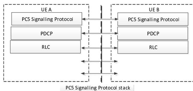
**Figure 23.10.2.2-2: Control-Plane protocol stack for one-to-one sidelink communication**
