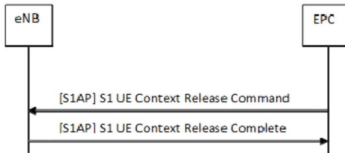
**Figure 19.2.2.2.1-1: S1 UE Context Release procedure (EPC triggered)**
