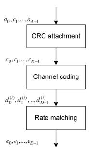
Figure 6.3.2-1: Transport block processing for UL-SCH
