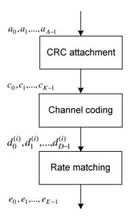
Figure 5.3.1-1: Transport channel processing for BCH
