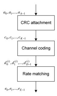
Figure 5.3.3-1: Processing for one DCI
