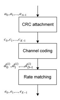
Figure 5.4.1-1: Transport channel processing for SL-BCH
