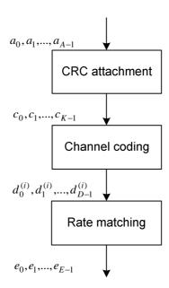
Figure 6.4.2-1: Transport block processing for DL-SCH and PCH
