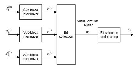
Figure 5.1.4-2. Rate matching for convolutionally coded transport channels and control information
