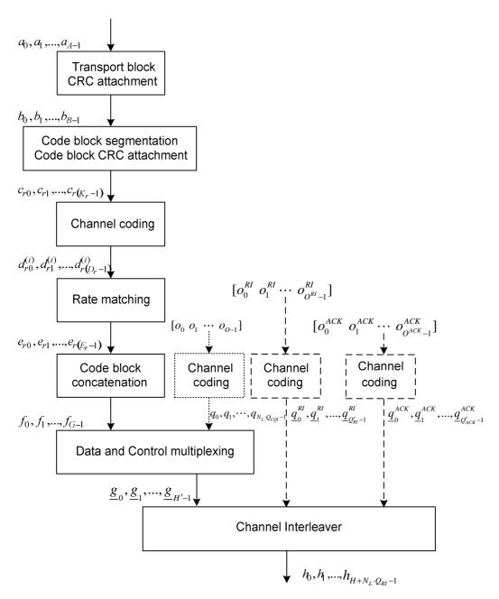
Figure 5.2.2-1: Transport block processing for UL-SCH
