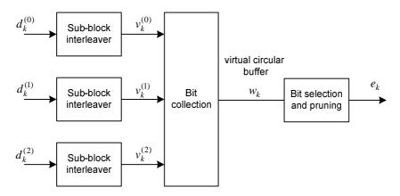
Figure 5.1.4-1. Rate matching for turbo coded transport channels
