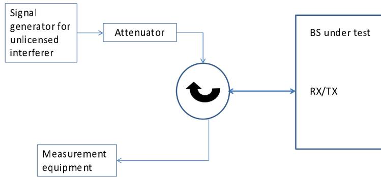
**Figure I.4: Measuring system Set-up for Channel access procedures**
