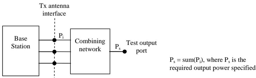
**Figure 4.5.7.2-1: Transmitter test set-up**
