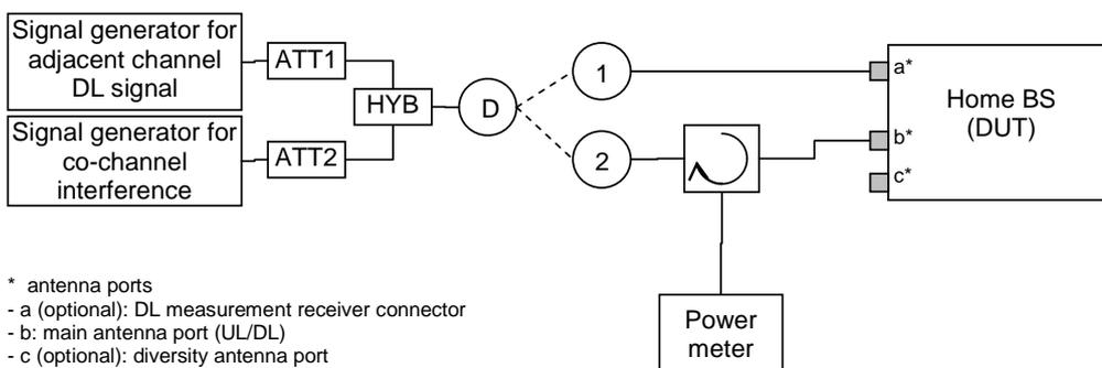
Figure I.1-4: Measuring system set-up for Home BS output power for adjacent channel protection
