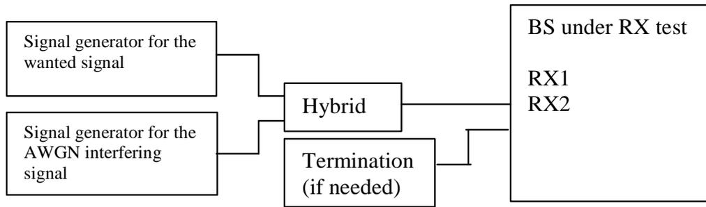
Figure I.2-2: Measuring system Set-up for Dynamic range
