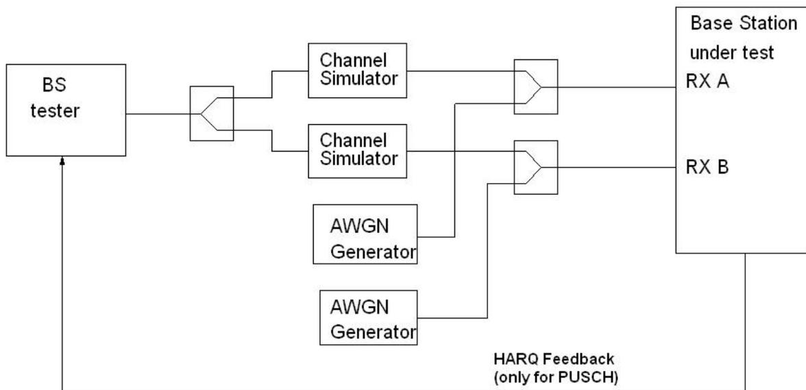
Figure I.3-2: Functional set-up for performance requirements for PUSCH, PRACH, single user PUCCH in multipath fading conditions and for High Speed Train conditions for BS with Rx diversity (2 Rx case shown)
