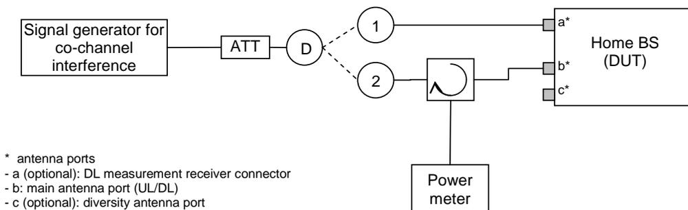
Figure I.1-5: (Option 1) Measuring system set-up for Home BS output power for co-channel E-UTRA protection
