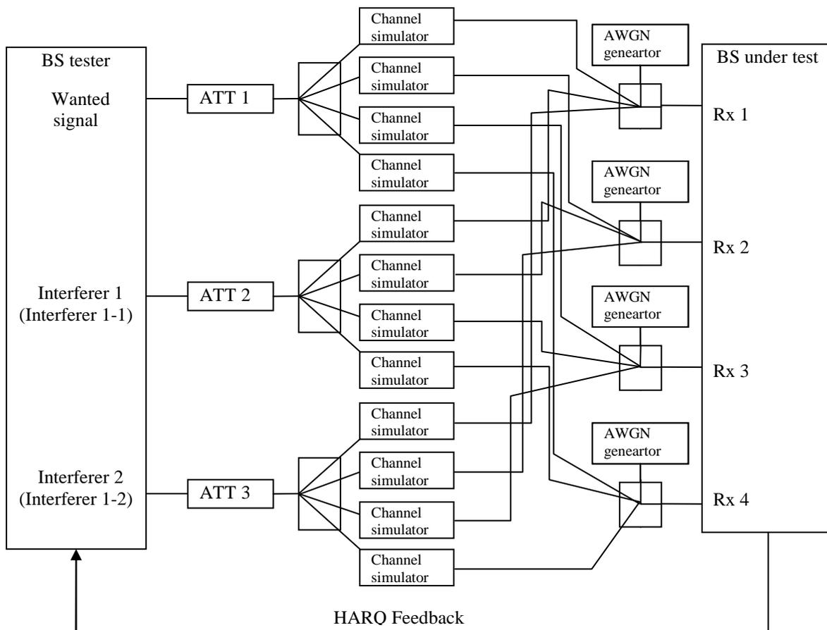
**Figure I.3-7c: Functional set-up for enhanced performance requirements type A of 4Rx PUSCH in multipath fading conditions with synchronous or asynchronous interference (2 interferers and 4 Rx case shown)**
