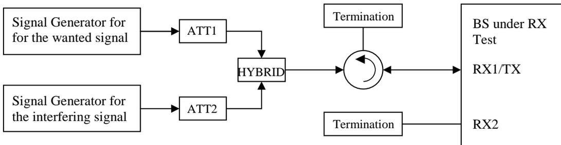
Figure I.2-5: Measuring system Set-up for Blocking characteristics
