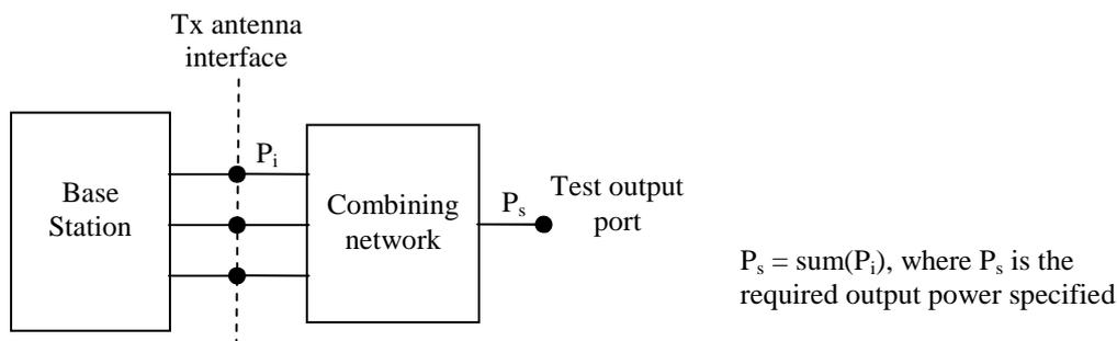
Figure 4.5.7.2-1: Transmitter test set-up
