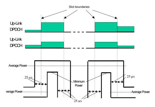
Figure 5.7.1: Transmit template during Compressed mode
