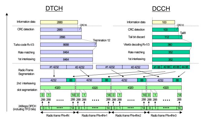
Figure C.3.3 (informative): Channel coding of DL reference measurement channel (144 kbps)
