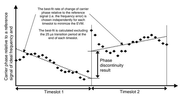
Figure 5.13.3.1 Graphical description of phase discontinuity
