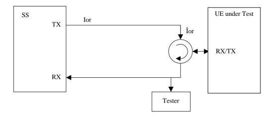
Figure A.1: Connection for Basic TX Test
