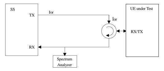
Figure A.8: Connection for Spurious Emission Test
