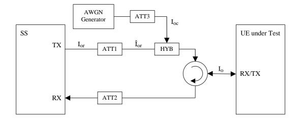
Figure A.9: Connection for Static Propagation Test
