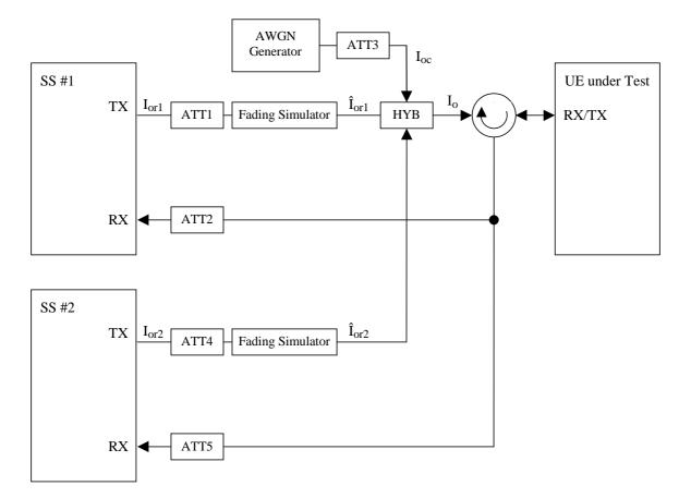
Figure A.11: Connection for Inter-Cell Soft Handover Test
