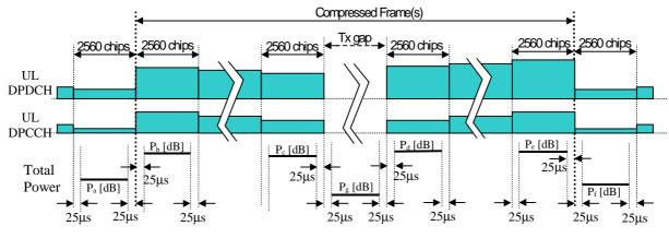
Figure 5.7.4: Uplink transmit power in uplink compressed mode
