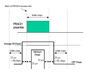
Figure 5.5.1: Transmit ON/OFF template for PRACH preambles
