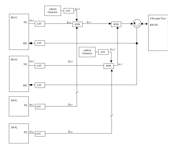
Figure A.15: Connection for cell reselection multi carrier multi cell
