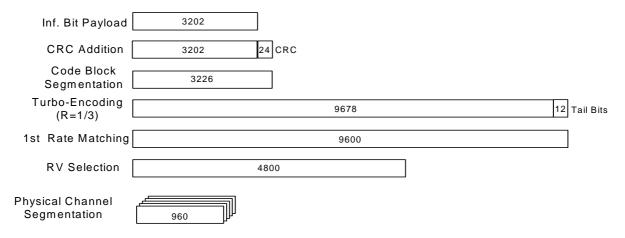
Figure C.8.1: Coding rate for Fixed reference Channel H-Set 1 (QPSK)
