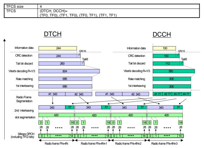
Table C.3.1.3: DL reference measurement channel, TFCS (12.2 kbps)
