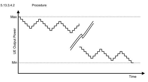
Figure 5.13.3.4 Five down four up hysteresis test pattern
