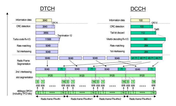
Figure C.3.4 (informative): Channel coding of DL reference measurement channel (384 kbps)
