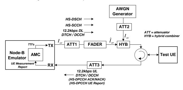
Figure A.17: Connection setup for HSDPA Reporting of Channel Quality Indicator
