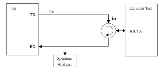
Figure A.8: Connection for Spurious Emission Test
