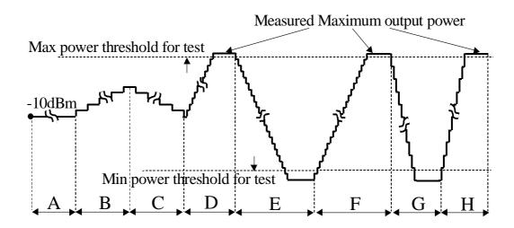
Figure 5.4.2.4 Inner Loop Power Control Test Steps
