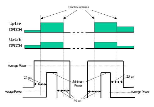
Figure 5.7.1: Transmit template during Compressed mode
