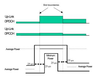
Figure 5.6.1: Transmit template during TFC change
