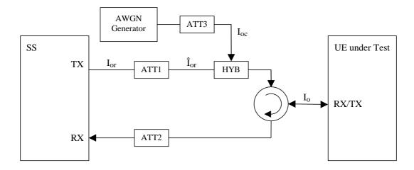
Figure A.9: Connection for Static Propagation Test
