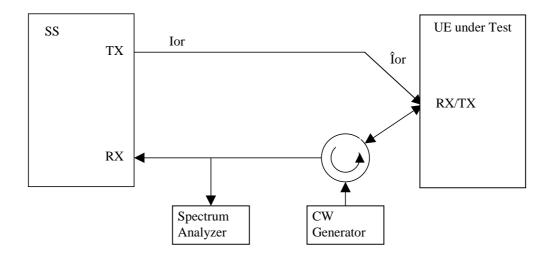
Figure A.2: Connection for TX Intermodulation Test
