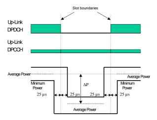
Figure 5.6.2: Transmit template during DTX
