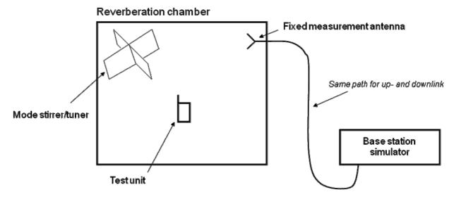
Figure A.2: A schematic picture of the reverberation chamber measurement setup.
