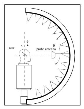
Figure A.1: The coordinate system used in the measurements for the head phantom
