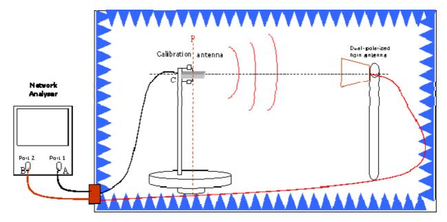
Figure B.1 Calibration/substitution procedures using a vector network analyzer.
