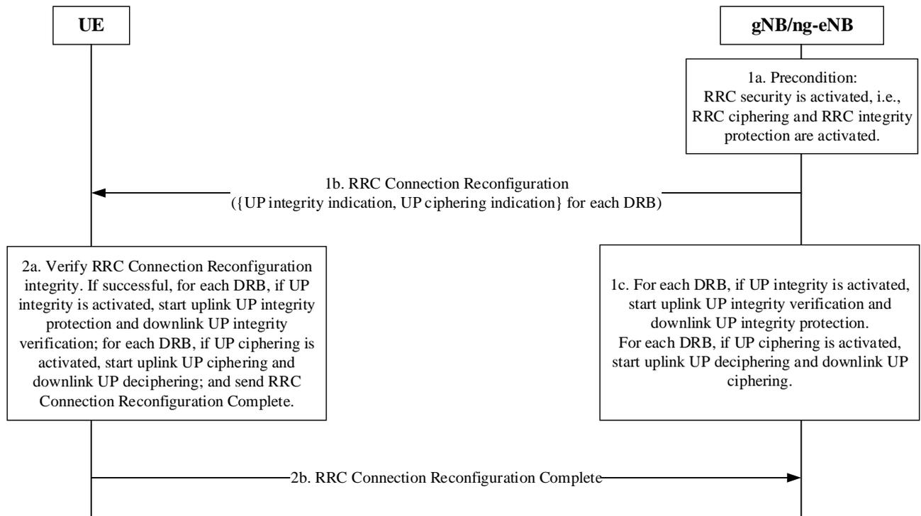
**Figure 6.6.2-1: User plane (UP) security activation mechanism**
