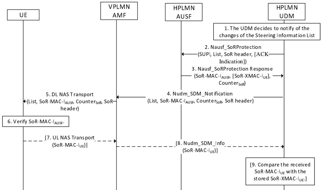
**Figure 6.14.2.2-1: Procedure for providing list of preferred PLMN/access technology combinations**
