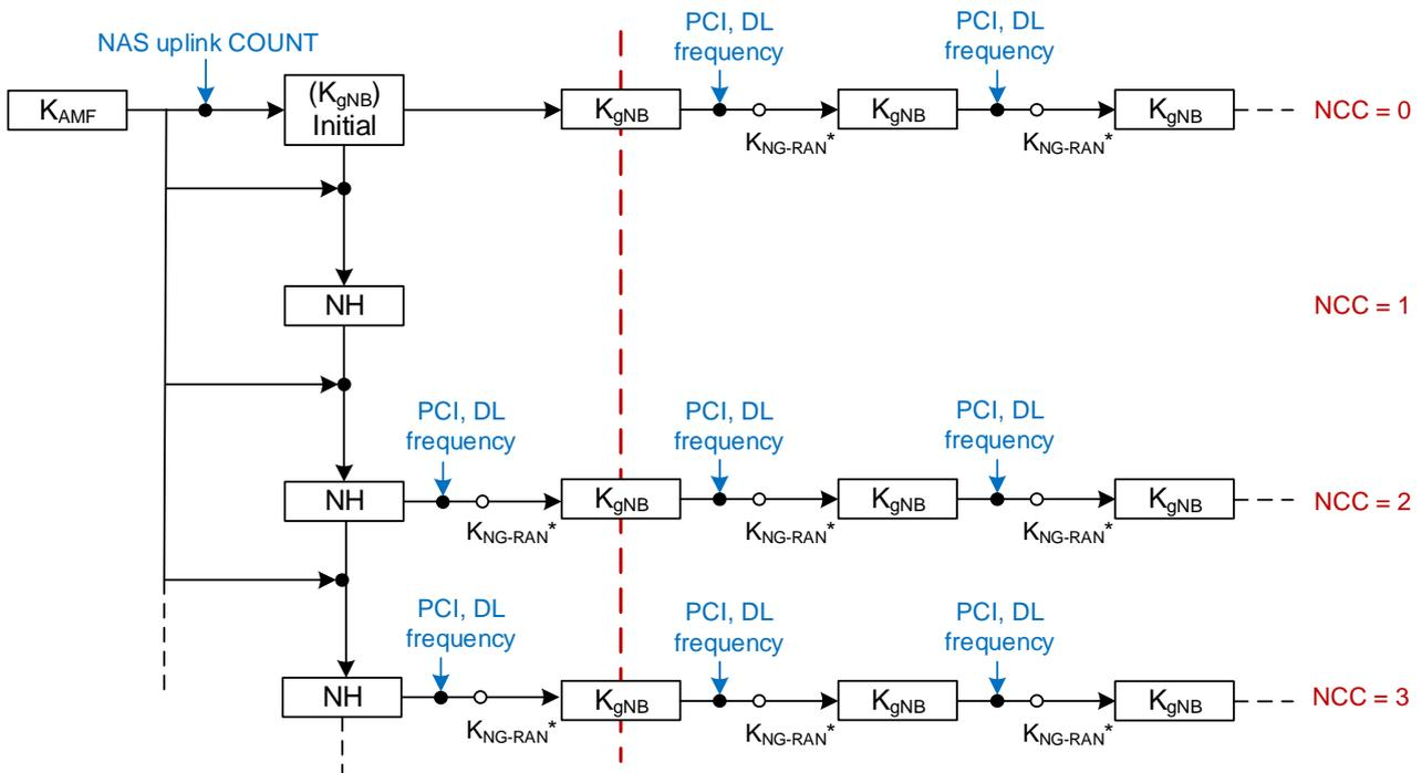
**Figure 6.9.2.1.1-1: Model for the handover key chaining**
