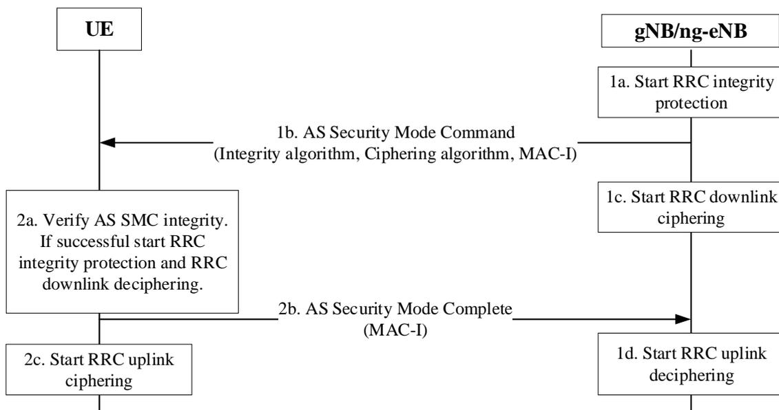
Figure 6.7.4-1: AS Security Mode Command Procedure
