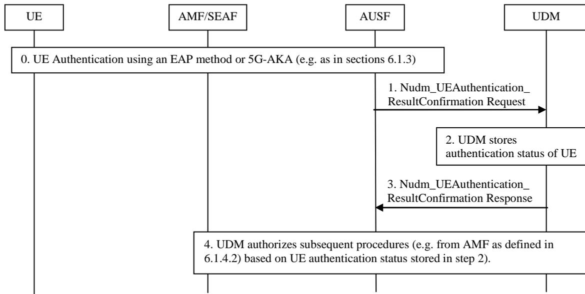
**Figure 6.1.4.1a-1: Linking increased Home control to subsequent procedures**
