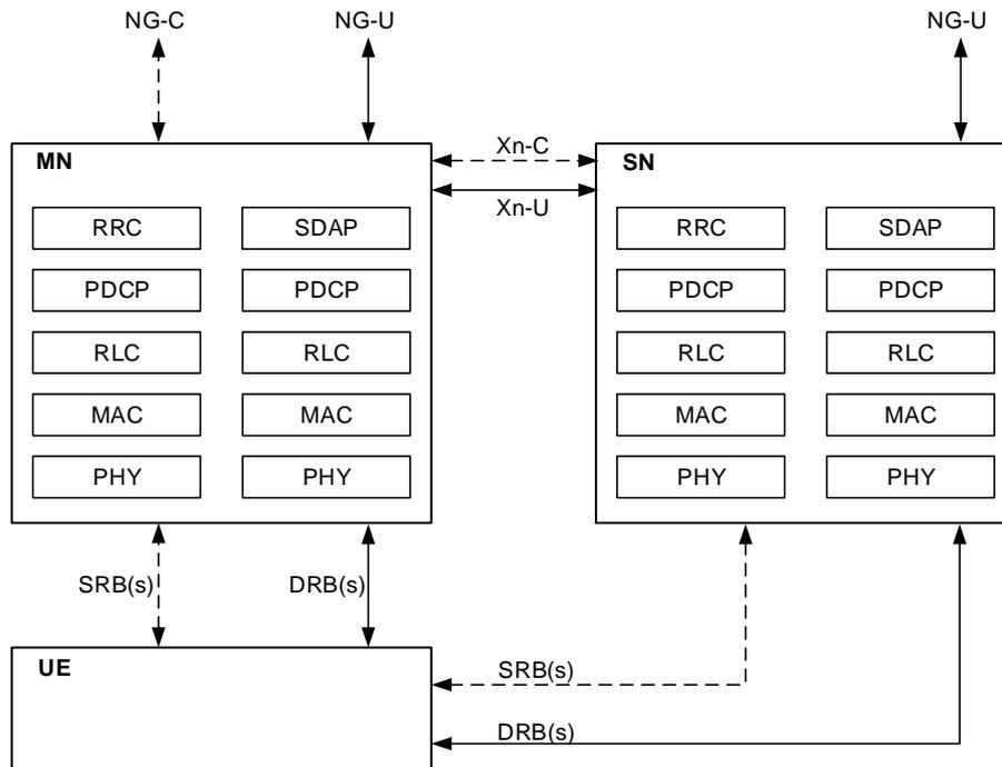
**Figure 6.10.1.2-1 Multi-Radio dual connectivity (MR-DC) protocol architecture.**
