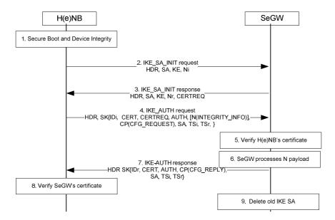
Figure A.1: Certificate-based authentication with device integrity
