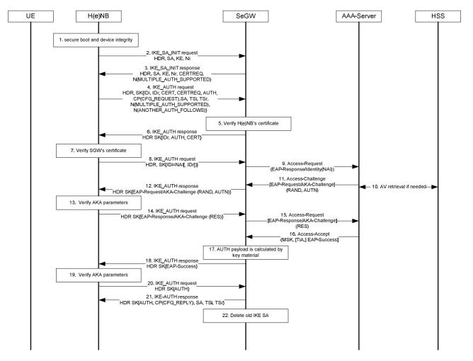
Figure A.2: Combined certificate and EAP-AKA-based authentication
