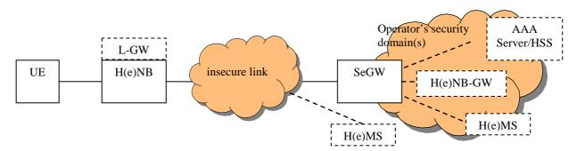
Figure 4.1.1: System Architecture of H(e)NB
