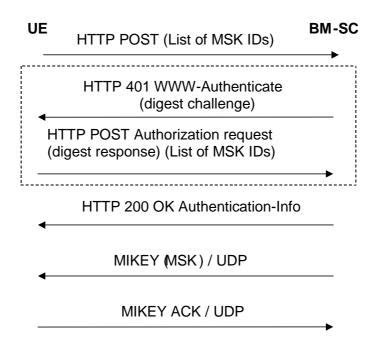
Figure 6.1: Basic MSK retrieval procedure
