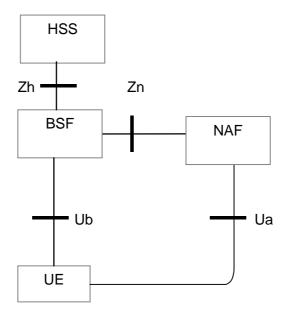
Figure 4.1: Simple network model for bootstrapping
