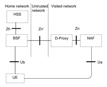
NOTE: The Zn' reference point is distinguished from the Zn reference point in that it is used between operators.
