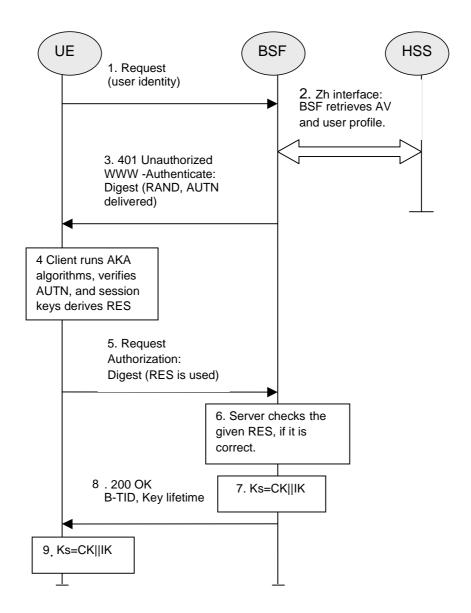
Figure 4.3: The bootstrapping procedure
