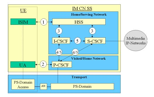
Figure 1: The IMS security architecture
