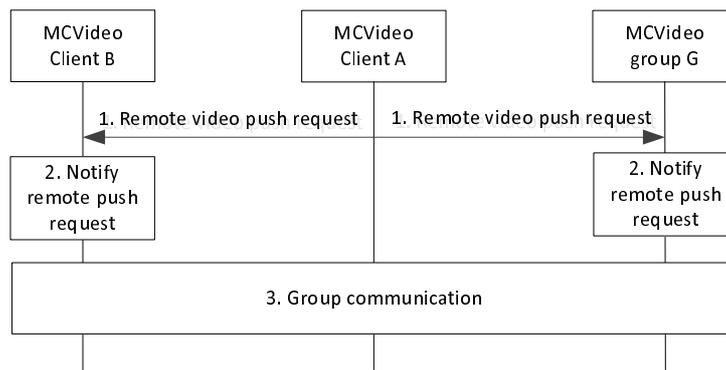
**Figure 7.3.11.1-2: Off-network remotely initiated video push to group**
