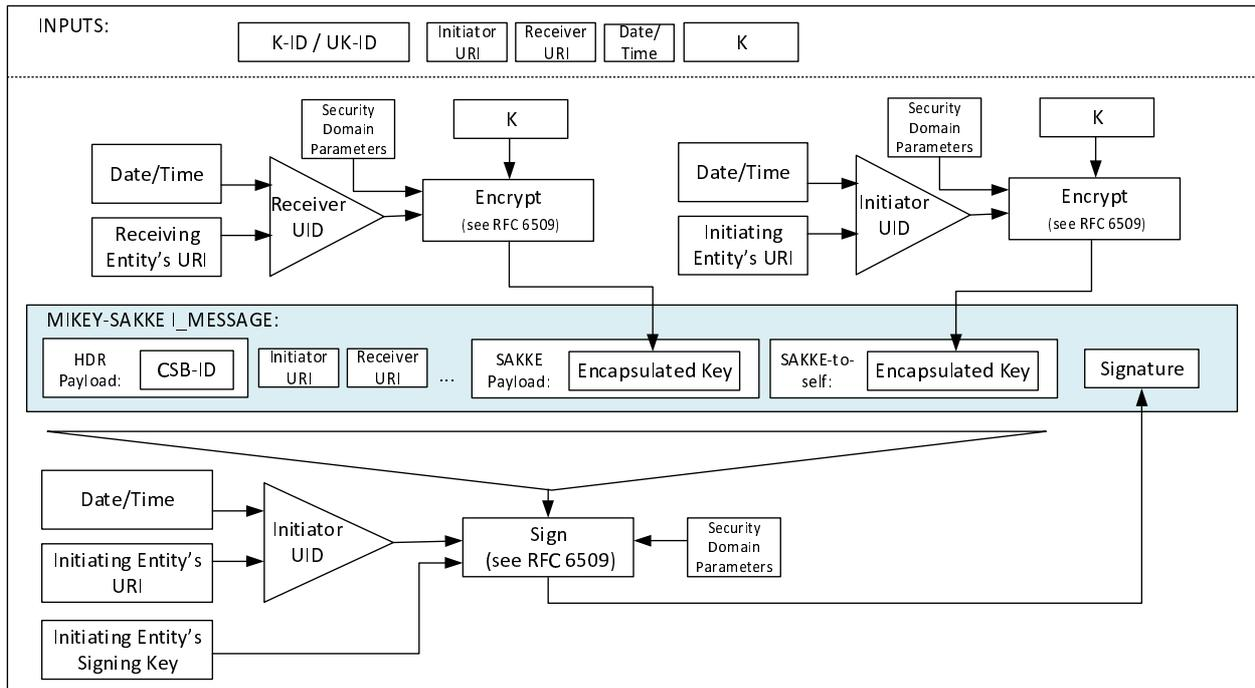
Figure 5.2.5-1: Common key distribution mechanism with SAKKE-to-self payload
