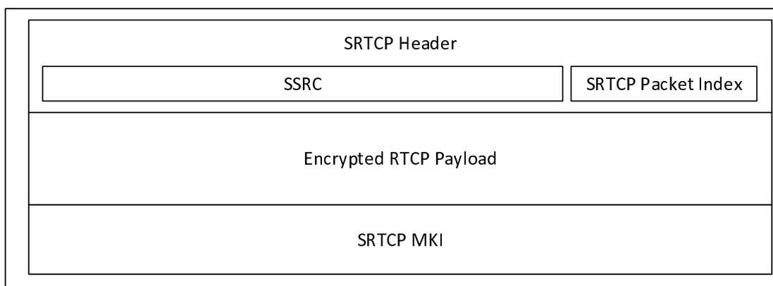
**Figure 9.4.7-2: SRTCP packet format showing security parameters**
