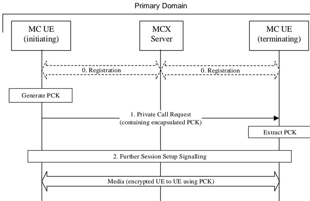
**Figure 7.2.2-1: Private call security procedure for on-network PCK distribution for single domain**
