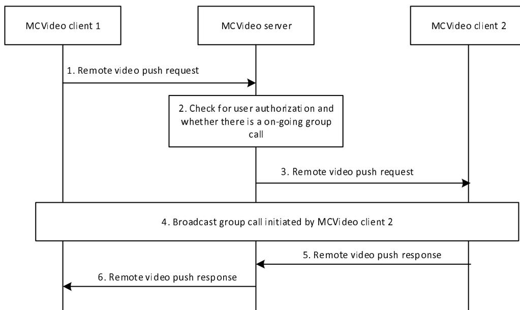
**Figure 7.3.11.1-1: On-network remotely initiated video push to group**
