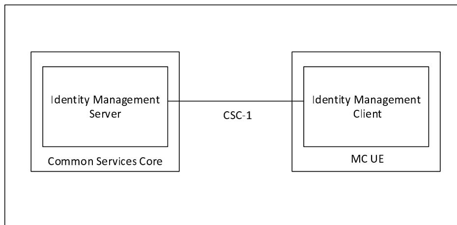
**Figure 5.1.2.1-1: Functional Model for MC Identity Management**
