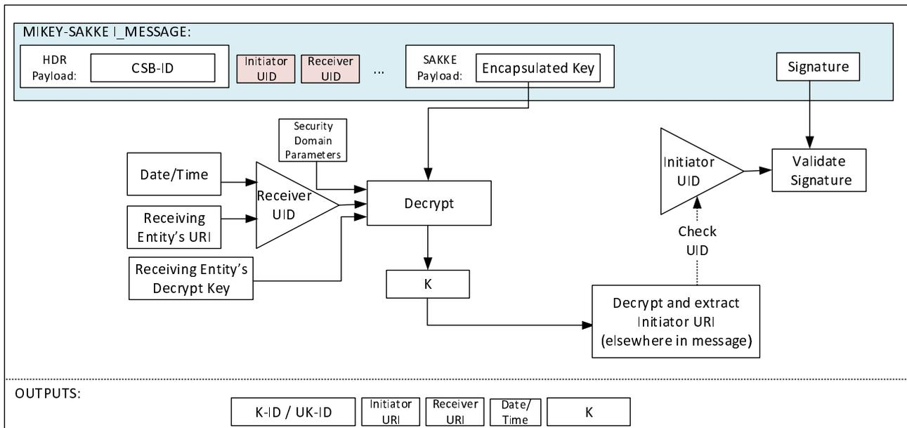
Figure 5.2.6-2: Common key extraction mechanism with identity hiding
