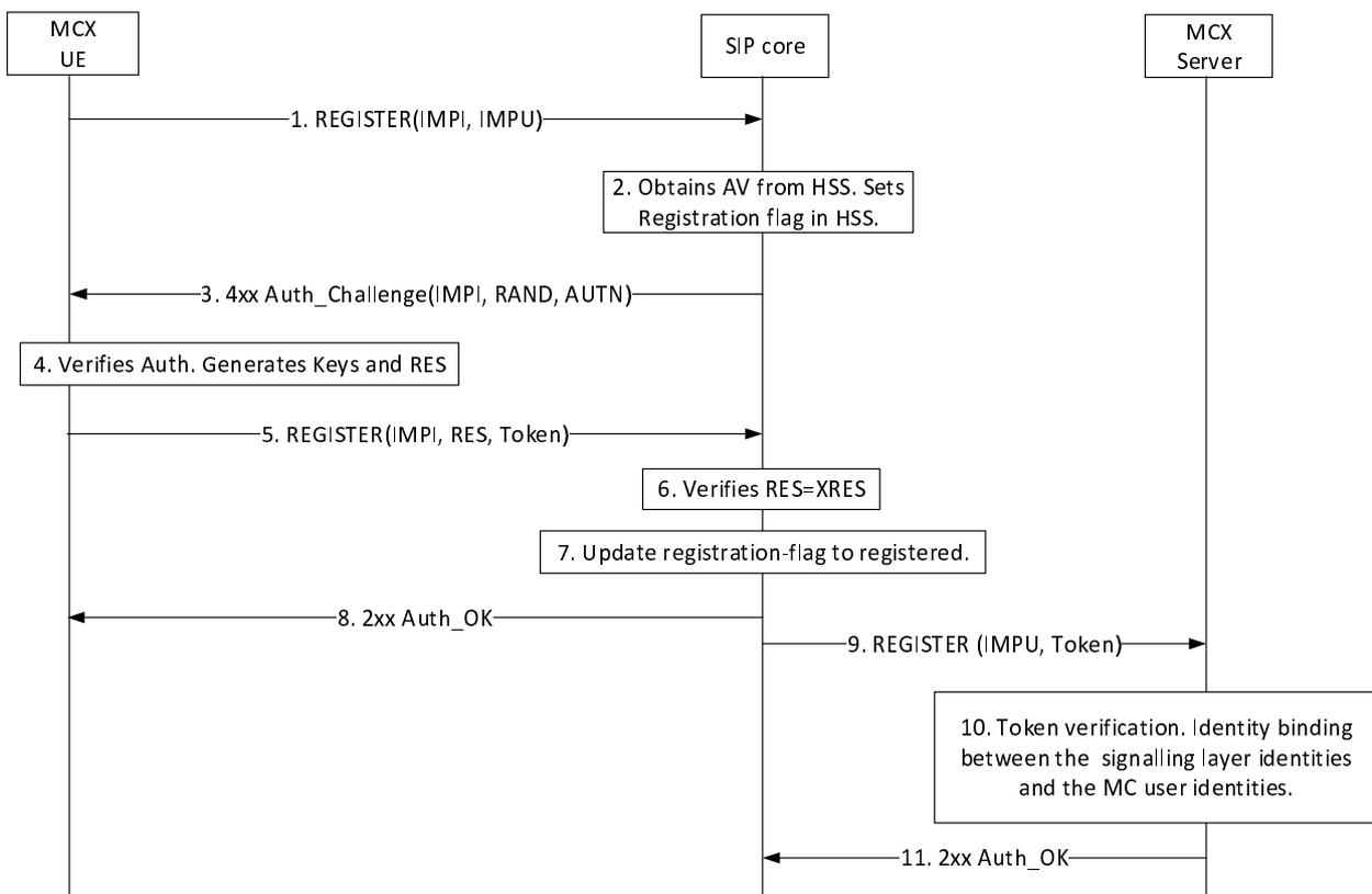
**Figure 5.1.3.2.2-1: MCX User Service Authorization using SIP REGISTER message**
