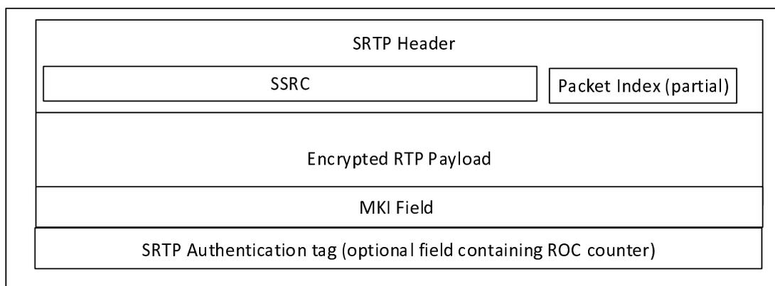
**Figure 7.5.2-2: SRTP packet format showing security parameters**
