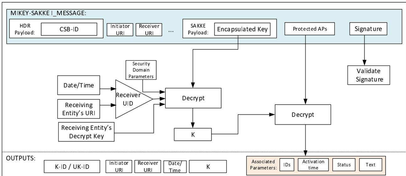
**Figure 5.2.4-2: Common key extraction mechanism with associated parameters**
