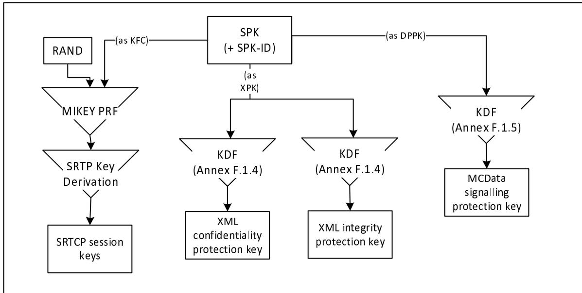
Figure 9.2.3-1: Uses of the Signalling Protection Key
