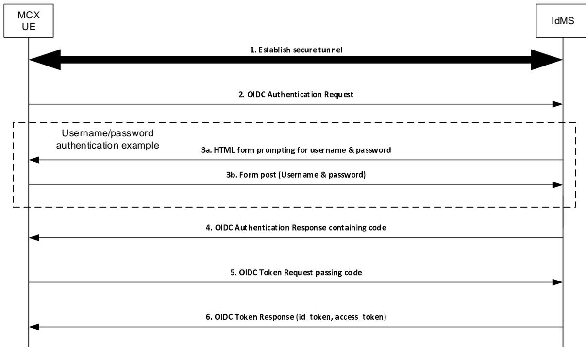
**Figure 5.1.2.3.2-1: OpenID Connect (OIDC) Example Using Username/Password**
