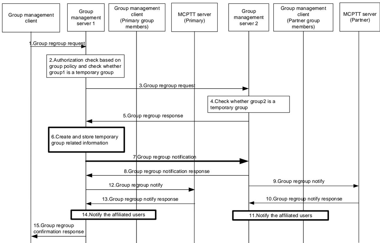
Figure 7.3.3.3-1: Group regroup security procedure (multiple MC domains)
