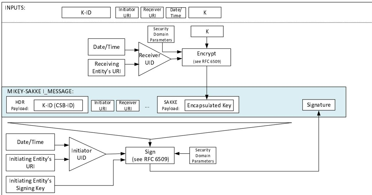
Figure 5.2.2-1: Common key distribution mechanism
