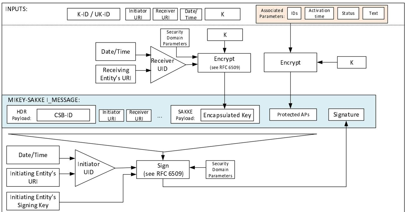
Figure 5.2.4-1: Common key distribution mechanism with associated parameters
