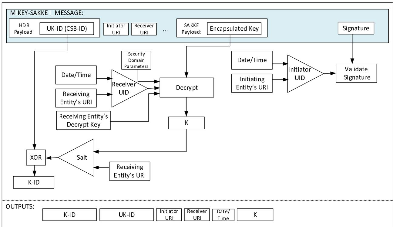
Figure 5.2.3-3: Common key extraction mechanism with end-point diversity
