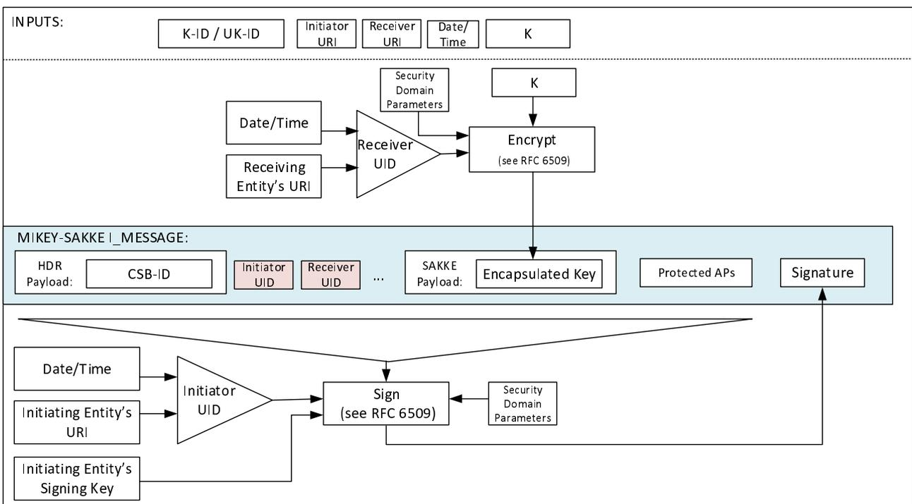
Figure 5.2.6-1: Common key distribution mechanism with identity hiding
