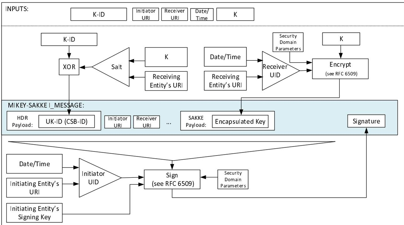
**Figure 5.2.3-2: Common key distribution mechanism with end-point diversity**
