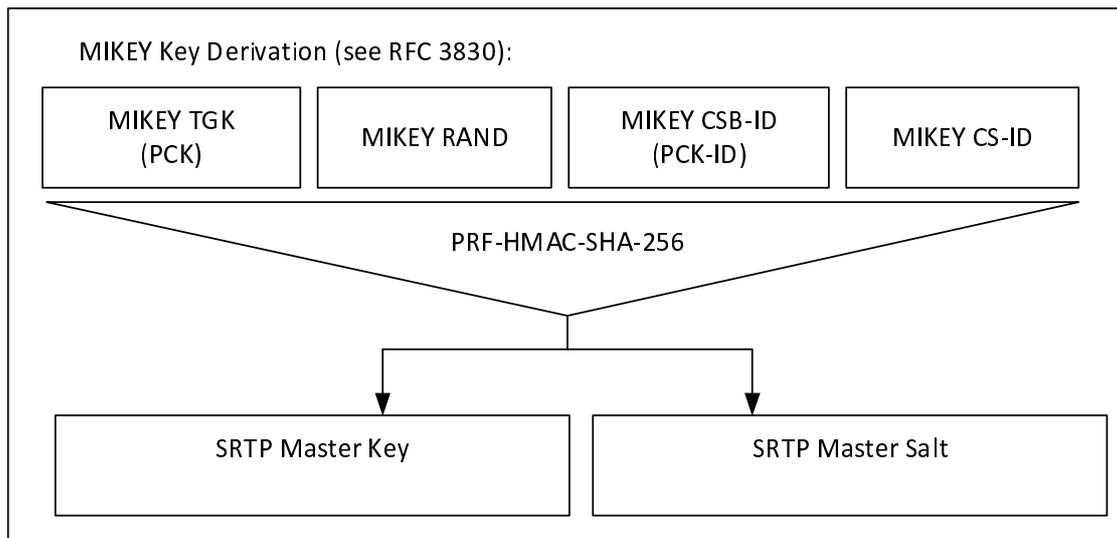
**Figure 7.4.1-1: Key Derivation for media stream protection**
