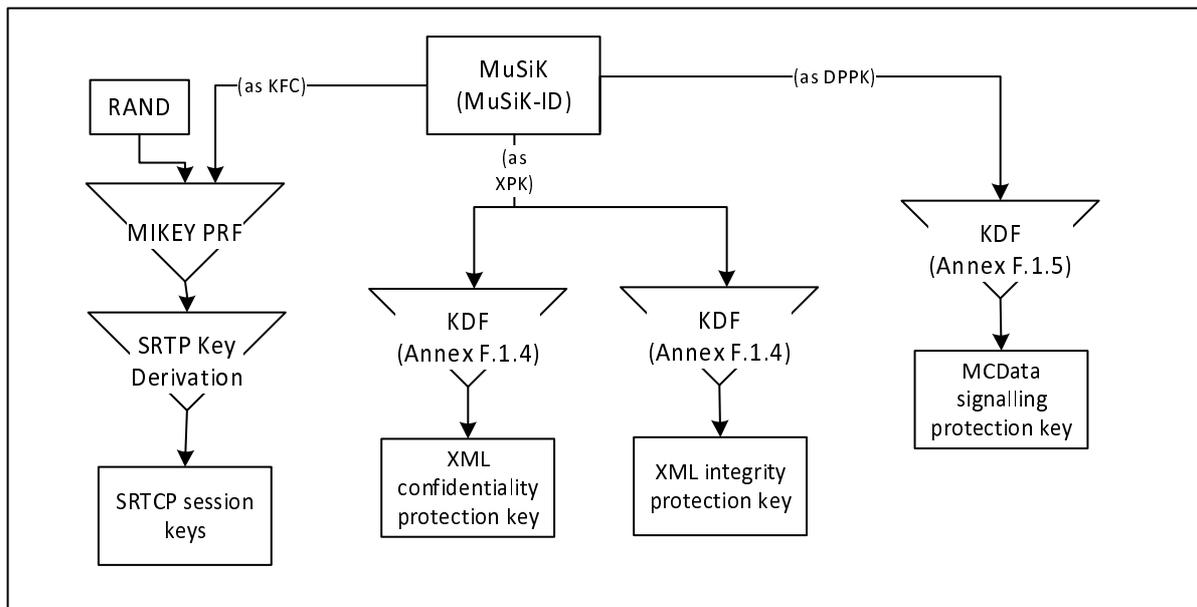
**Figure 9.2.2-1: Uses of the Multicast Signalling Key (MuSiK)**
