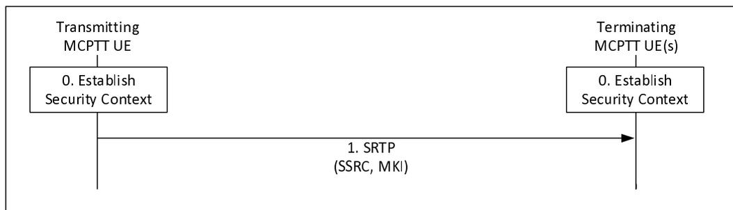
**Figure 7.5.2-1: Security procedure for media stream protection**
