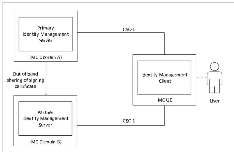
**Figure 5.1.4.2-1: Functional Model for Inter-Domain MC Identity Management**
