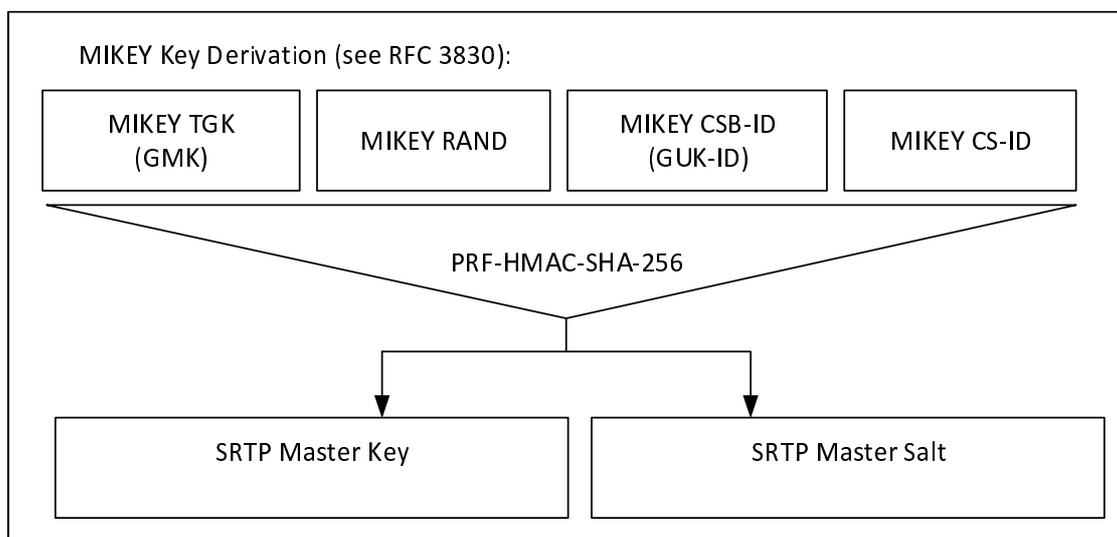
**Figure 7.4.2-1: Key Derivation for media stream protection**
