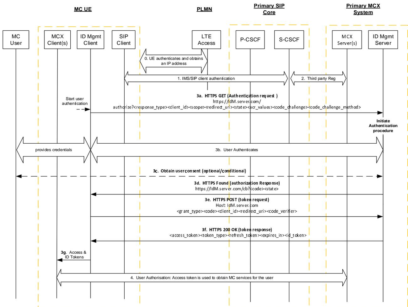
**Figure C.1-1: OpenID Connect MC User Authentication and Registration**
