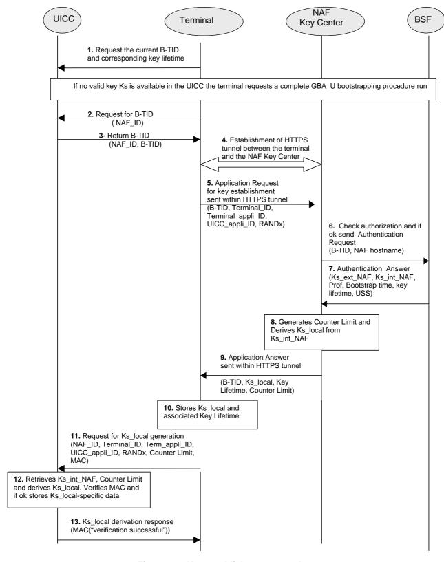
Figure 4-3: Key establishment procedure
