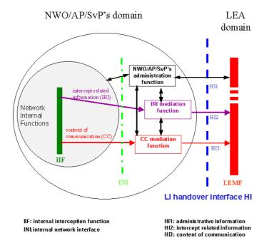
Figure 4.1: Functional block diagram showing handover interface HI
