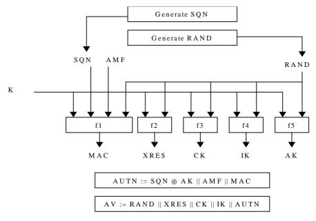
Figure 4: Generation of an authentication vector
