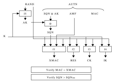
Figure 2: User authentication function in the USIM
