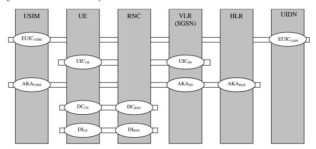
Figure 1: UMTS functional security architecture
