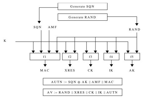
Figure 4: Generation of an authentication vector
