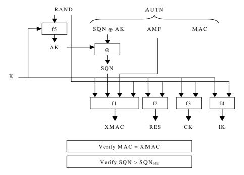
Figure 2: User authentication function in the USIM
