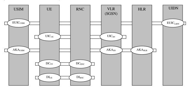
Figure 1: UMTS functional security architecture
