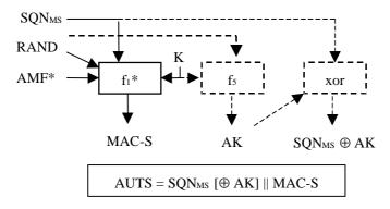
Figure 3: Generation of a token for re-synchronisation AUTS (note 1)
