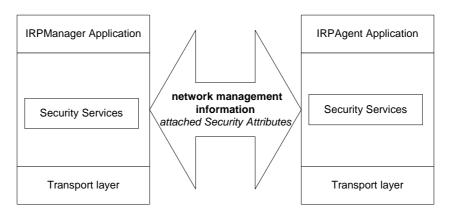
Figure B.1 : Principles of IRP Security Service
