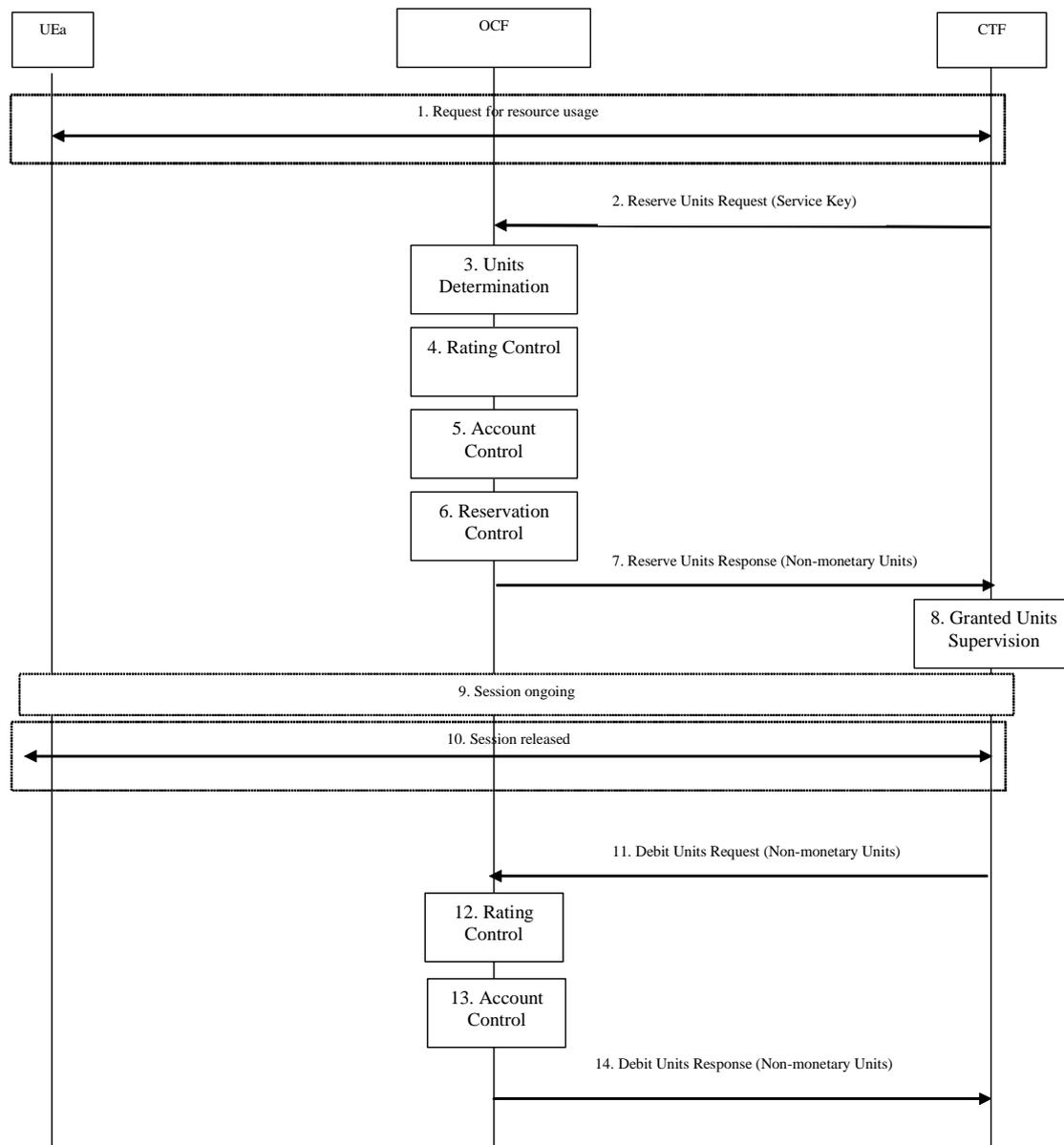
**Figure 5.2.2.3.2: Session Charging with Reservation / Centralized Unit Determination and Centralized Rating**
