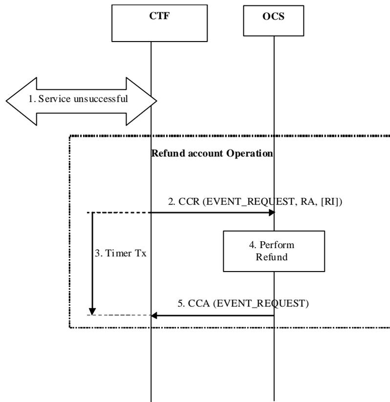
**Figure 6.3.3a: IEC Direct Debiting Operation for refund purpose**
