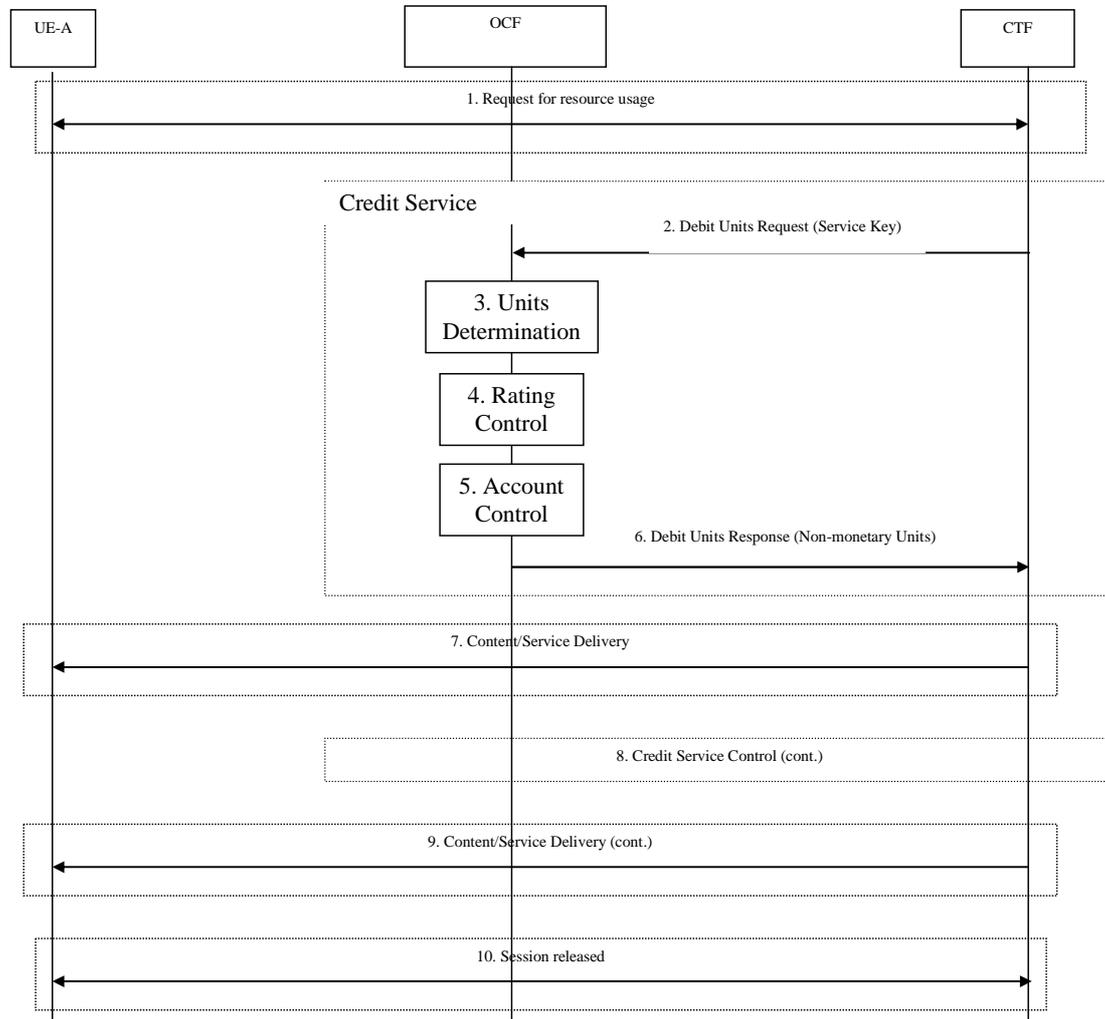
**Figure 5.2.2.1.2: Immediate Event Charging with Centralized Rating and Centralized Unit Determination**
