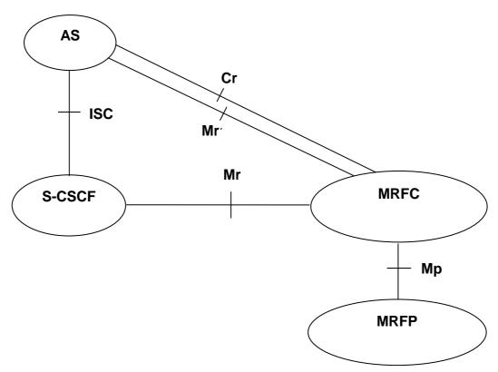
Figure 4.2.1: Architecture of Media Resource Function in IMS
