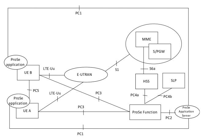
Figure 4.1.1: Non-roaming reference architecture
