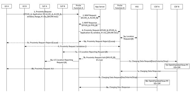
Figure 5.2.2.2.1: Message flow for ProSe EPC-level Discovery Proximity Request
