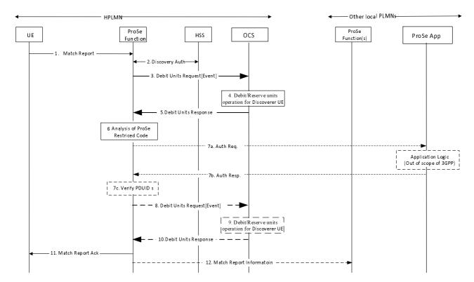
Figure 5.3.2.2.6.1: Match Report procedure for Model B restricted discovery (IEC for non-roaming)
