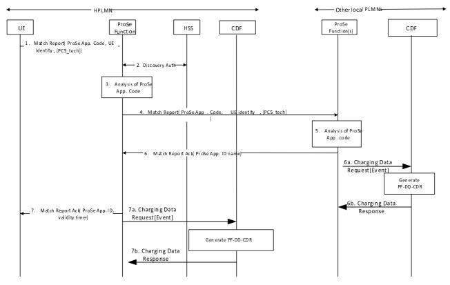
Figure 5.2.2.1.4.1: Message flow for Match Report of Open Discovery (non-roaming)
