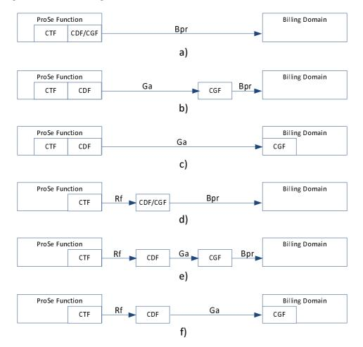
Figure 4.2.1: ProSe offline charging architecture
