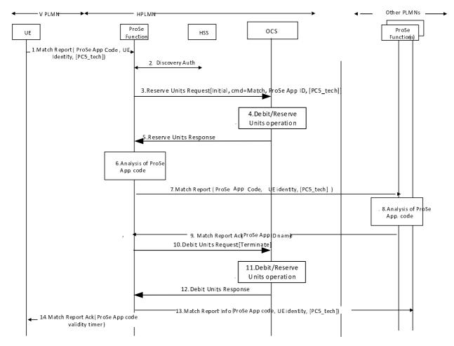
Figure 5.3.2.2.4.4: Message flow for ProSe Direct Open Discovery Match Report Request (ECUR for roaming/ inter-PLMN transmission)
