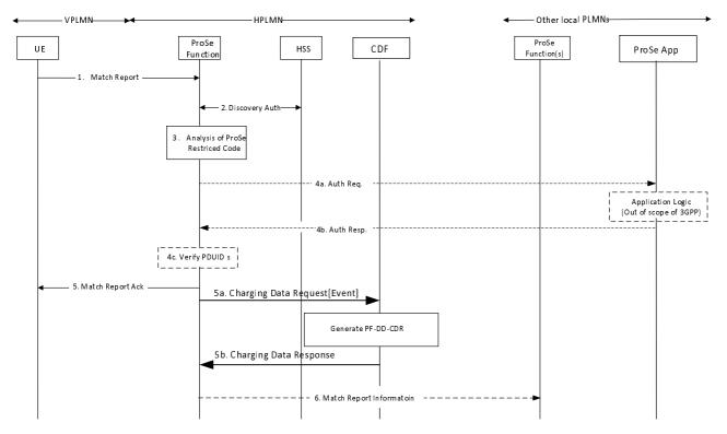
Figure 5.2.2.1.4.3: Message flow for Match Report of Restricted Discovery (roaming//inter-PLMN transmission)
