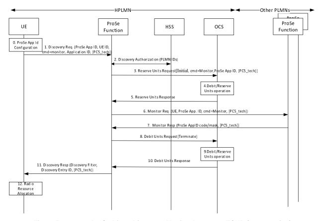
Figure 5.3.2.2.3.2: ProSe Direct Discovery Monitor Request – ECUR (non-roaming)
