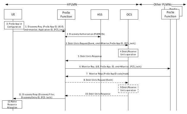
Figure 5.3.2.2.3.1: ProSe Direct Discovery Monitor Request – IEC (non-roaming)
