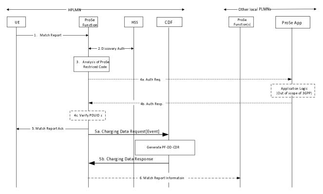
Figure 5.2.2.1.4.1A: Message flow for Match Report of Restricted Discovery (non-roaming)
