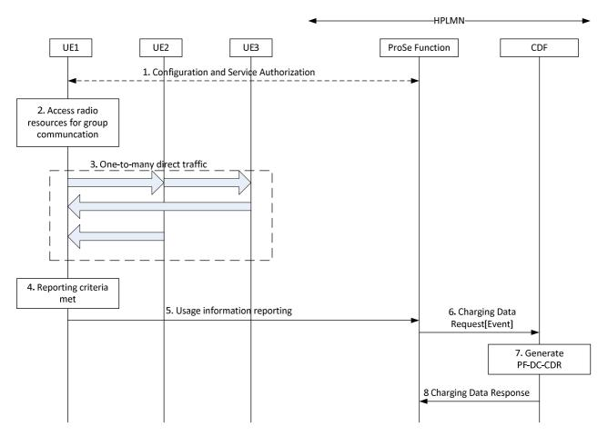
Figure 5.2.2.3.2.1: Offline Charging for ProSe one-to-many Direct Communication
