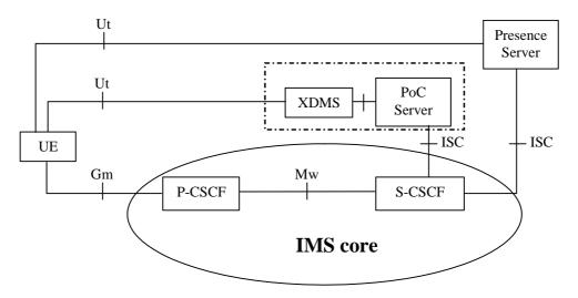
Figure 4.1.1: PoC service elements in the IMS architecture
