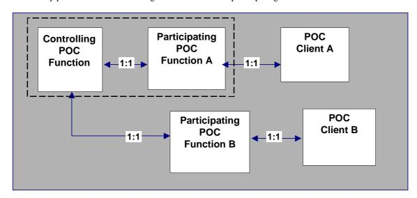
Figure 4.1.1.2.1: Relationship between controlling PoC function, participating PoC functions and the PoC Clients for 1-1 PoC session in a single network
