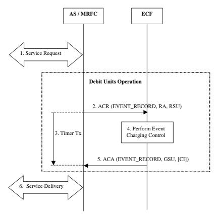
Figure 6.1: IEC - Debit Units Operation
