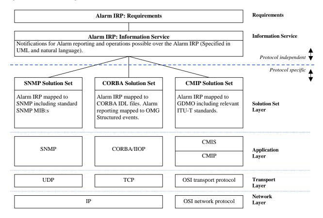
Figure 4.4: Example of an IRP (Alarm IRP)
