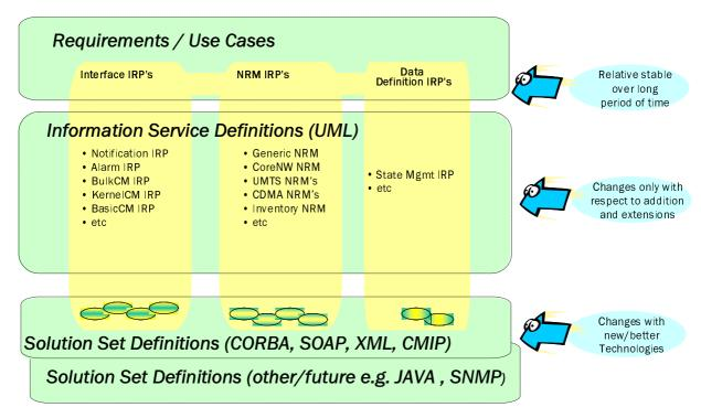
Figure 4.2: The IRP 3-Level Specifications Approach combined with the three IRP categories.
