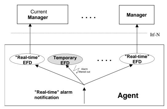
Figure 2: Treatment of "real time" alarms
