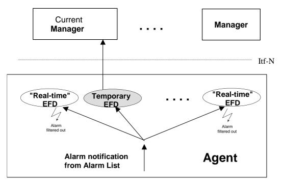
Figure 3: Treatment of "alignent" alarms
