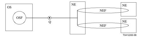
Figure A.1: Distributed network element
