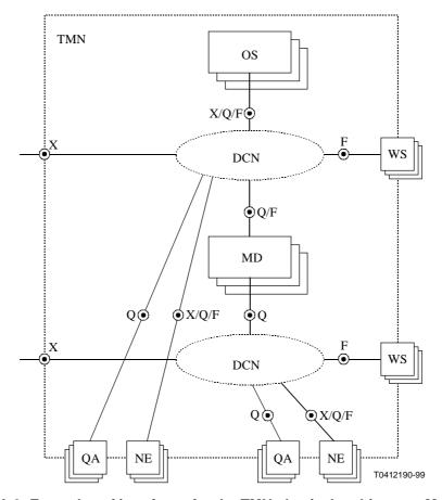
Figure A.2: Examples of interfaces for the TMN physical architecture M.3010 [1]
