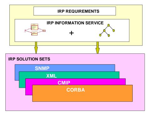
Figure 10.1: IRP components (with example solution sets)
