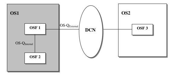
Figure 8.4: Operations Systems intra-operability Architecture
