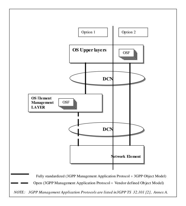
Figure 8.1: Network Element Management Architecture
