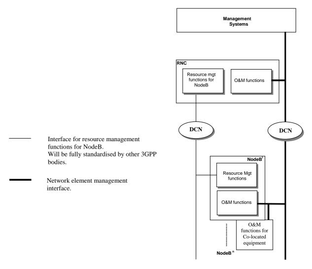
Figure 5: Network and Subnetwork Management Architecture
