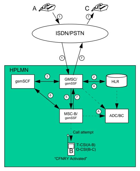
Figure B.15: Incoming call handled by CAMEL without redirection and forwarded late using GSM SS but controlled by CAMEL
