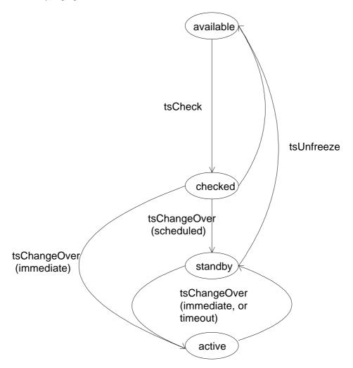
Figure A.6: Tariff system state transition diagram
