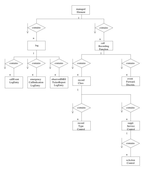
Figure A.3: The call recording view
