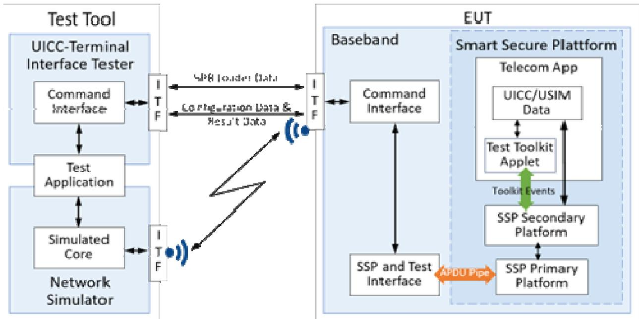
Figure 4.5: Test environment for UEs with ETSI eSSP/iSSP
