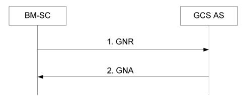
Figure A.1.3-1: TMGI Expiry Notification Procedure
