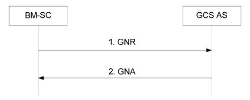
Figure A.2.4-1: MBMS Bearer Status Indication Procedure
