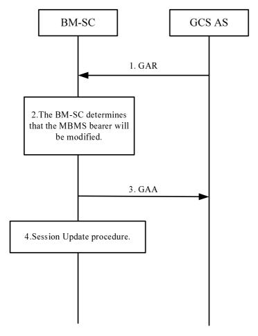
Figure A.2.3.1: Modify MBMS bearer Procedure
