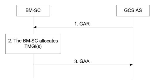
Figure A.1.1-1: TMGI Allocation Procedure
