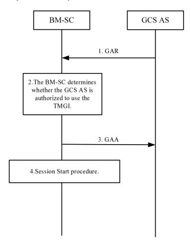
Figure A.2.1.1: Activate MBMS bearer Procedure
