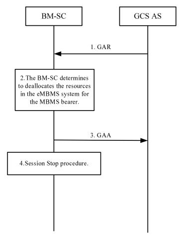
Figure A.2.2.1: Deactivate MBMS bearer Procedure
