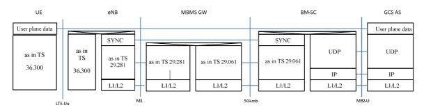
Figure 7.1-1: The user plane protocol stack without security protocols on the MB2-U reference point and in the EPC
