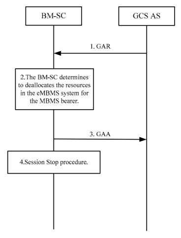
Figure A.2.2.1: Deactivate MBMS bearer Procedure
