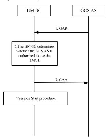
Figure A.2.1.1: Activate MBMS bearer Procedure
