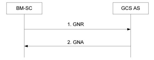
Figure A.1.3-1: TMGI Expiry Notification Procedure
