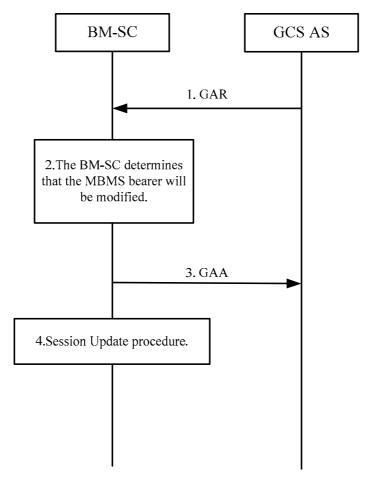
Figure A.2.3.1: Modify MBMS bearer Procedure
