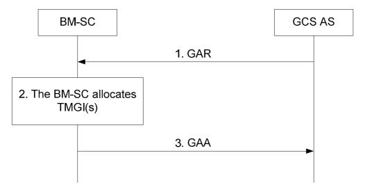
Figure A.1.1-1: TMGI Allocation Procedure
