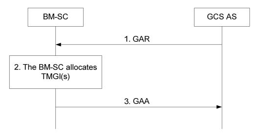
Figure A.1.1-1: TMGI Allocation Procedure
