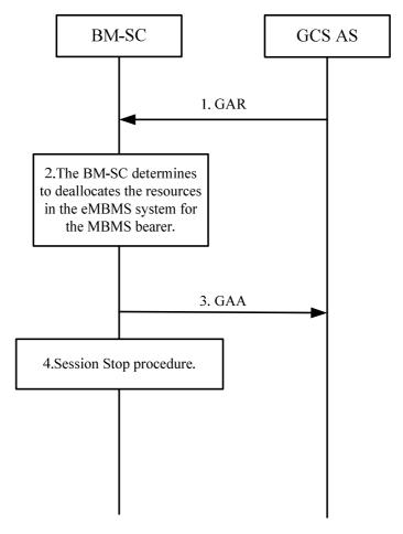
Figure A.2.2.1: Deactivate MBMS bearer Procedure
