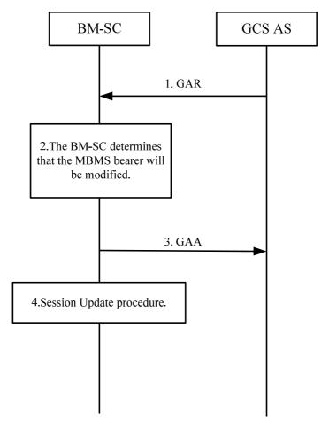
Figure A.2.3.1: Modify MBMS bearer Procedure
