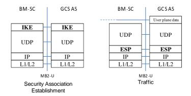
Figure 7.1-3: MB2-U Protocol stack with IPSec Security without UDP encapsulation
