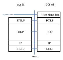
Figure 7.1-2: MB2-U Protocol stack with DTLS Security
