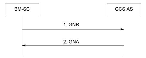
Figure A.2.4-1: MBMS Bearer Status Indication Procedure
