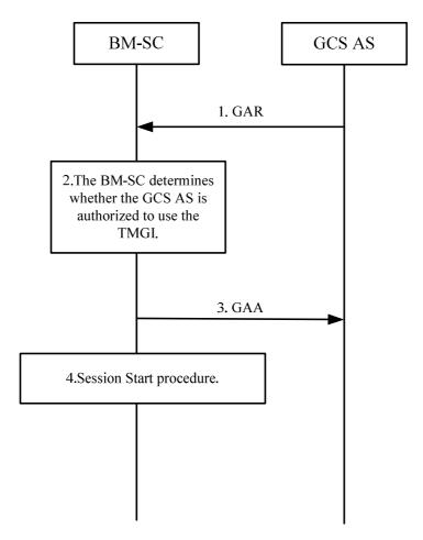
Figure A.2.1.1: Activate MBMS bearer Procedure
