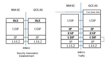
Figure 7.1-4: MB2-U Protocol stack with IPSec Security with UDP encapsulation
