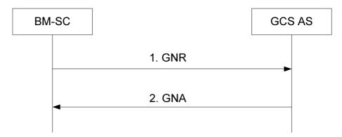
Figure A.1.3-1: TMGI Expiry Notification Procedure
