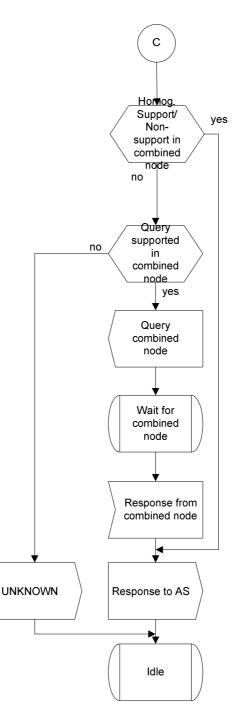
When receiving a T-ADS request from an Application Server, the HSS checks whether serving nodes (i.e. SGSN and/or MME) are registered (i.e. GPRS services and/or EPS services are actually subscribed, serving node addresses are stored and not marked as purged).
