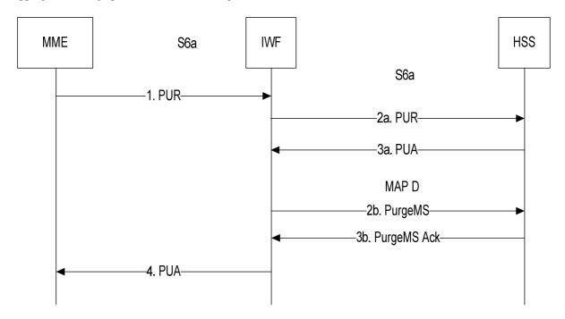
Figure A.4.4.1: Mapping of the Purge procedure
