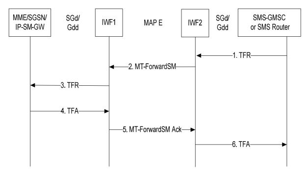
Figure A.2.4.2.2-1: Mapping of MT Forward Short Message procedure with two IWFs
