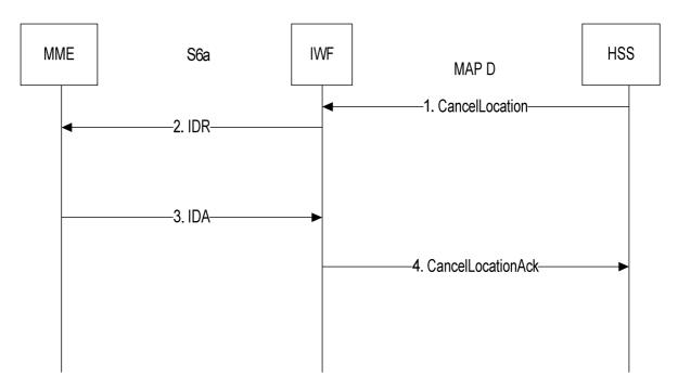
Figure A.4.4.3.2-1: Mapping of the Cancel Location over MAP D procedure
