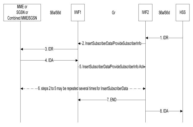
Figure 7.5.2-1: Mapping of Insert Subscriber Data Procedure for scenario with two IWFs
