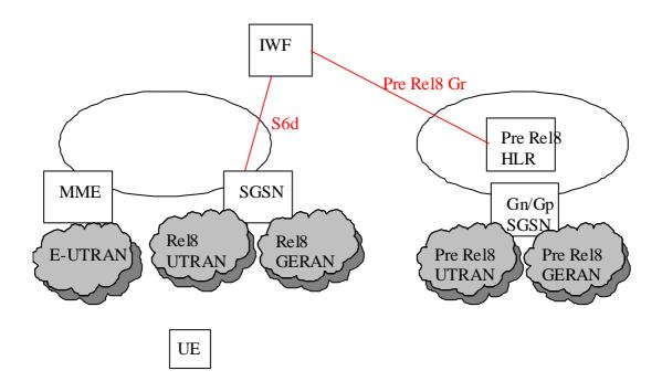
Figure 4.2.2-2 IWF Scenario one network deployment: visited EPS with E-UTRAN and UTRAN/GERAN, home Pre Rel8 UMTS/GPRS only
