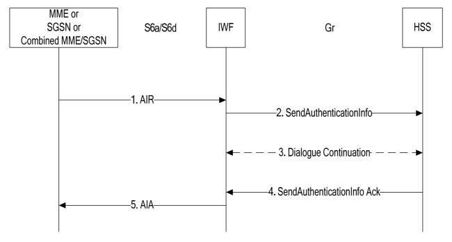
Figure 7.1.1-1: Mapping of Authentication Info Retrieval Procedure for scenario with one IWF
