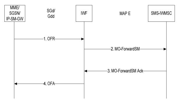
Figure A.2.4.1.1-1: Mapping of MO Forward Short Message procedure with one IWF
