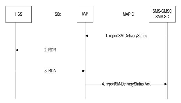
Figure A.3.4.3-1: Mapping of Report SM Delivery Status procedure
