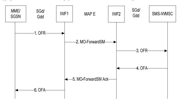
Figure A.2.4.1.2-1: Mapping of MO Forward Short Message procedure with two IWFs
