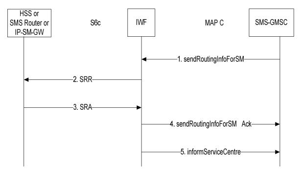
Figure A.3.4.1-1: Mapping of Send Routing Info for SM procedure
