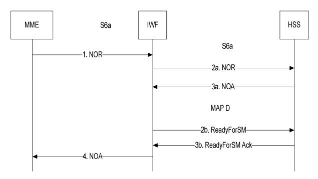
Figure A.4.4.8-1: Mapping of the Notification Procedure
