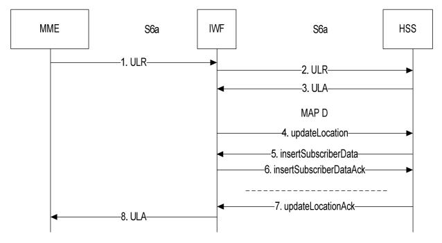
Figure A.4.4.2-1: Mapping of the Update Location procedure
