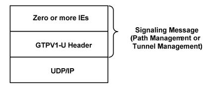
Figure: 4.4-2 Signalling Message Protocol Stack
