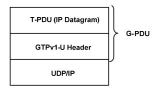
Figure: 4.4-1 G-PDU Protocol Stack
