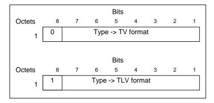
Figure 8.1-1: Type field for TV and TLV format
