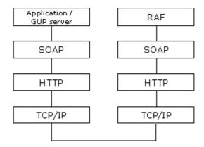
Figure 7.7.2 GUP Rp reference point protocol architecture
