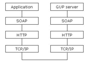
Figure 7.2.1 GUP Rg reference point protocol architecture
