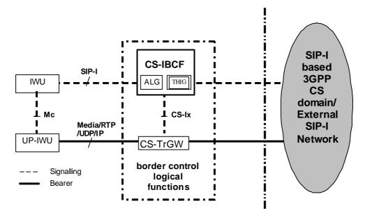
Figure A.3.1: CS-IBCF and CS-TrGW in SIP-I based CS domain
