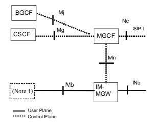
NOTE 1: The IM-MGW may be connected via the Mb to various network entities, such as a UE (via a GTP Tunnel to a GGSN), an MRFP, a TrGW or an AGW.
