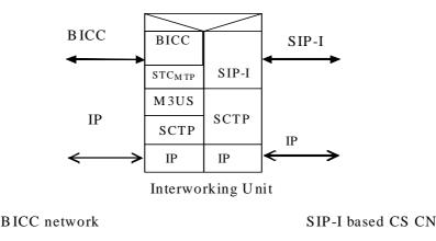
Figure 6.2.2.1: Control plane interworking between SIP-I based CS CN and a BICC based network with IP signalling transport
