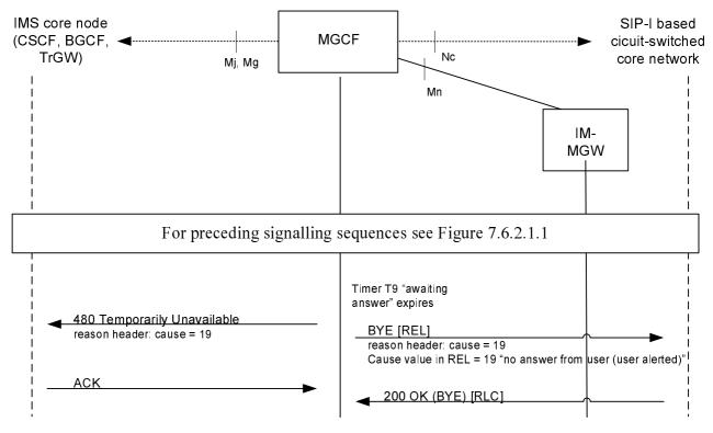
Figure 7.6.2.2.1: Incoming Call Failure (message sequence chart), called subscriber does not answer
