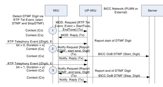
Figure 6.7.2.2: DTMF interworking: SIP-I to BICC, implicit duration (message sequence chart)
