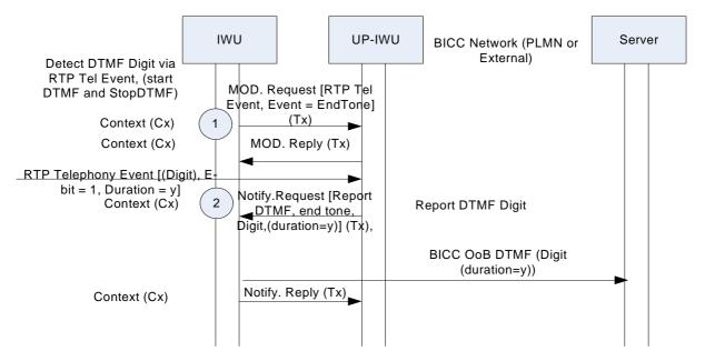
Figure 6.7.2.1: DTMF interworking: SIP-I to BICC, explicit duration (message sequence chart)
